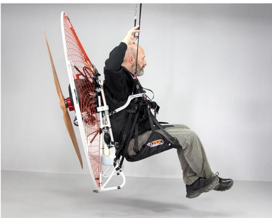
The paramotor thrust line angle with the engine OFF should be between 15 to 25 degrees
