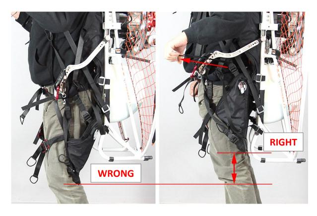
Adjust this strap to raise the harness seat plate to a parallel position between your body and the paramotor frame. **Test this in standing and sitting position (simulator)**
