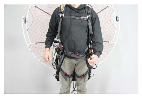
This strap should be closed in flight to allow the ASC bars to work in parallel
