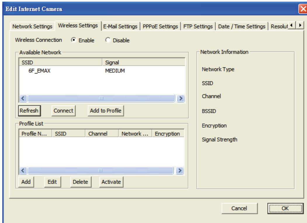
Utility will site survey automatically or you can press “Refresh” button to survey the AP router manually.
