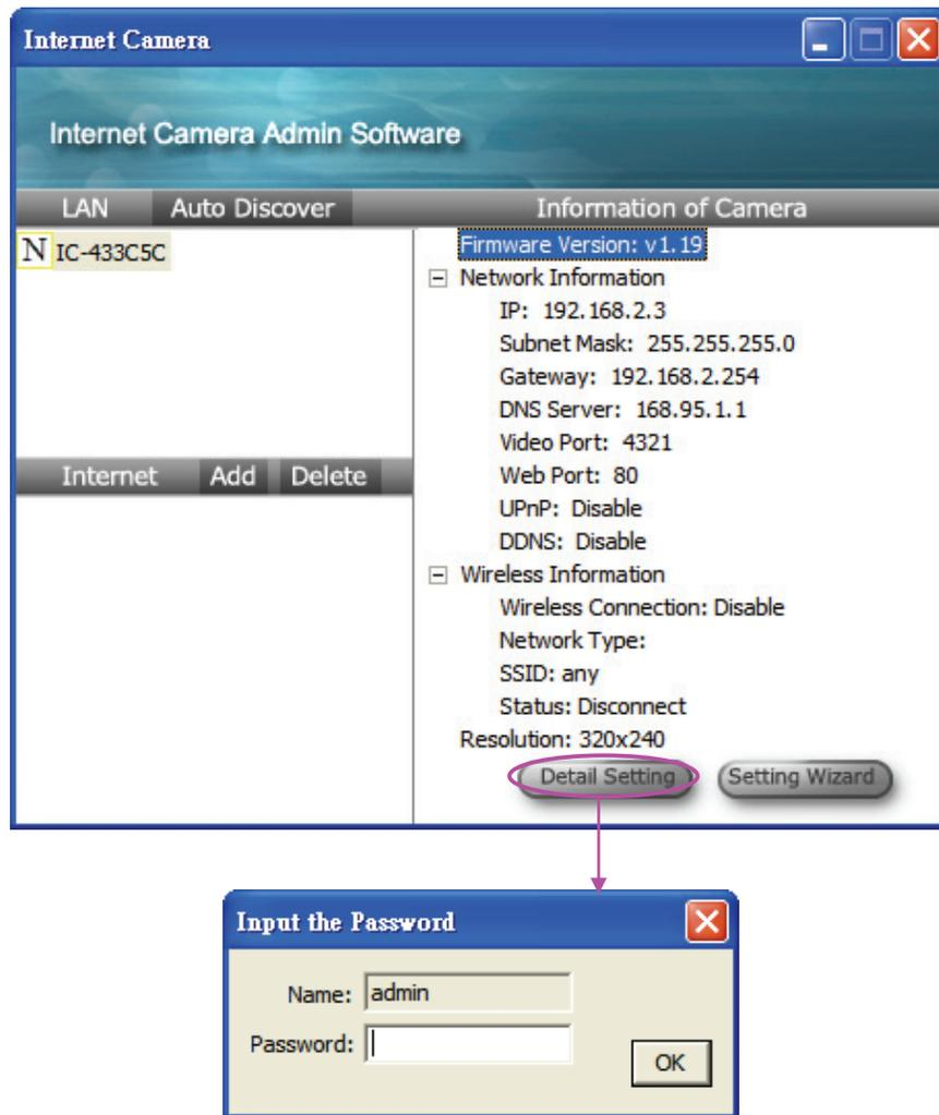
If the name and password you enter are correct, you can start to setup the camera.
