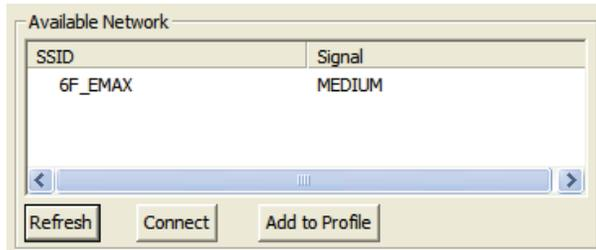
Then press “Connect” to connect AP router or press “Add to Profile” to configure the Wireless WEP and WPA encryption.
