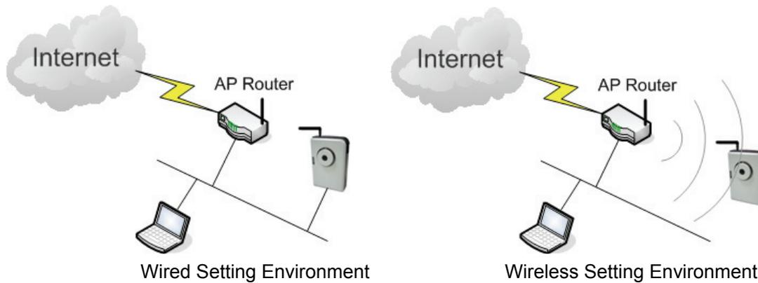
**You must configure the wireless settings from wired environment. Then you can remove the wired cable and start wireless connection.**
