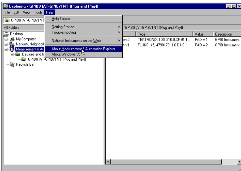
**Figure 2-11.** Select About Measurement & Automation Explorer
