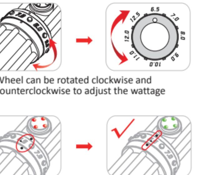
The red LED will blink six times and turn off if the rotational wheel is not in place.
