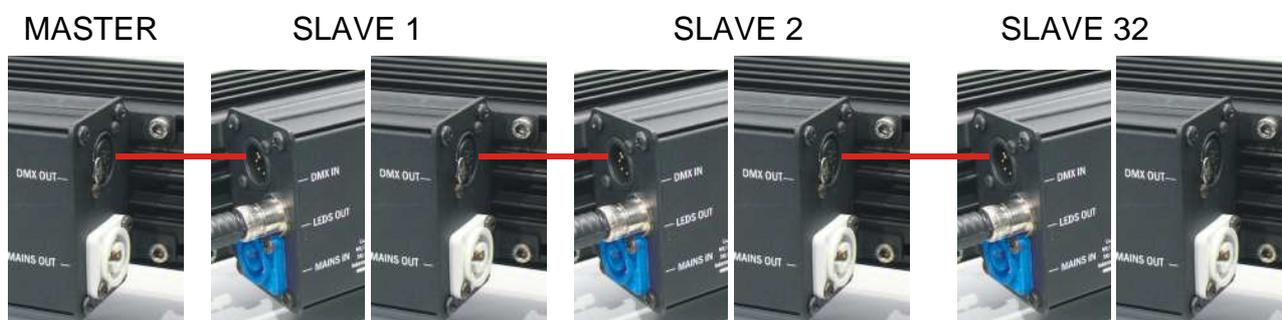
To activate Auto mode on the first unit, use the menu to run through the different modes until AUTO appears on the display, and press enter.
