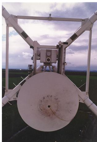
Fig. 3.2 : Primary focus feed positioner
