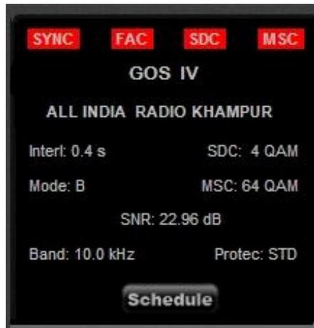
If DRM is selected as demodulation mode, the “DRM Info Panel” is activated. It displays some information about the DRM transmission. Clicking on **Schedule** button, if an internet connection is available, the software automatically downloads and displays the last DRM schedule from <ftp://216.92.35.131>.
