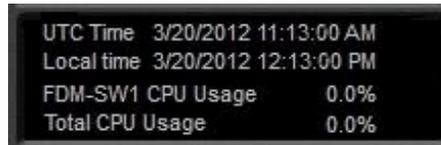
This panel displays the system time (UTC and local) and the CPU usage.
