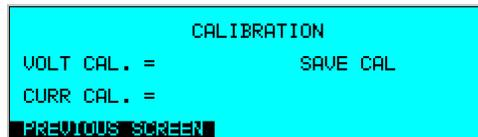
To adjust the calibration of voltage and current, enter the external reference reading in the corresponding field using the numeric keypad and press the ENTER key. The 3091LD will perform a measurement and adjust its calibration scale factors to match the external reference reading entered. Once both parameters have been calibrated, it is important to save the new scale factors in Flash EPROM memory. To do so, move the cursor to the SAVE CAL field and press ENTER.
