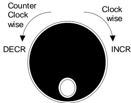
The shuttle knob is located to the right of the LCD screen and is used to change setup parameters. Note that it cannot be used to move the cursor position between menu fields. Use the UP and DOWN arrow keys in the FUNCTION keypad for this.
