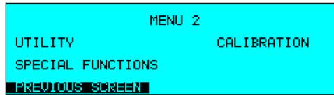
To access the CALIBRATION screen, press the MENU key twice to display the MENU 2 screen. Press the ↑ or ↓ key several times to highlight CALIBRATION. Press the ENTER key. The will display the password entry screen which prevents unauthorized access to the calibration parameters of the AC Load.
