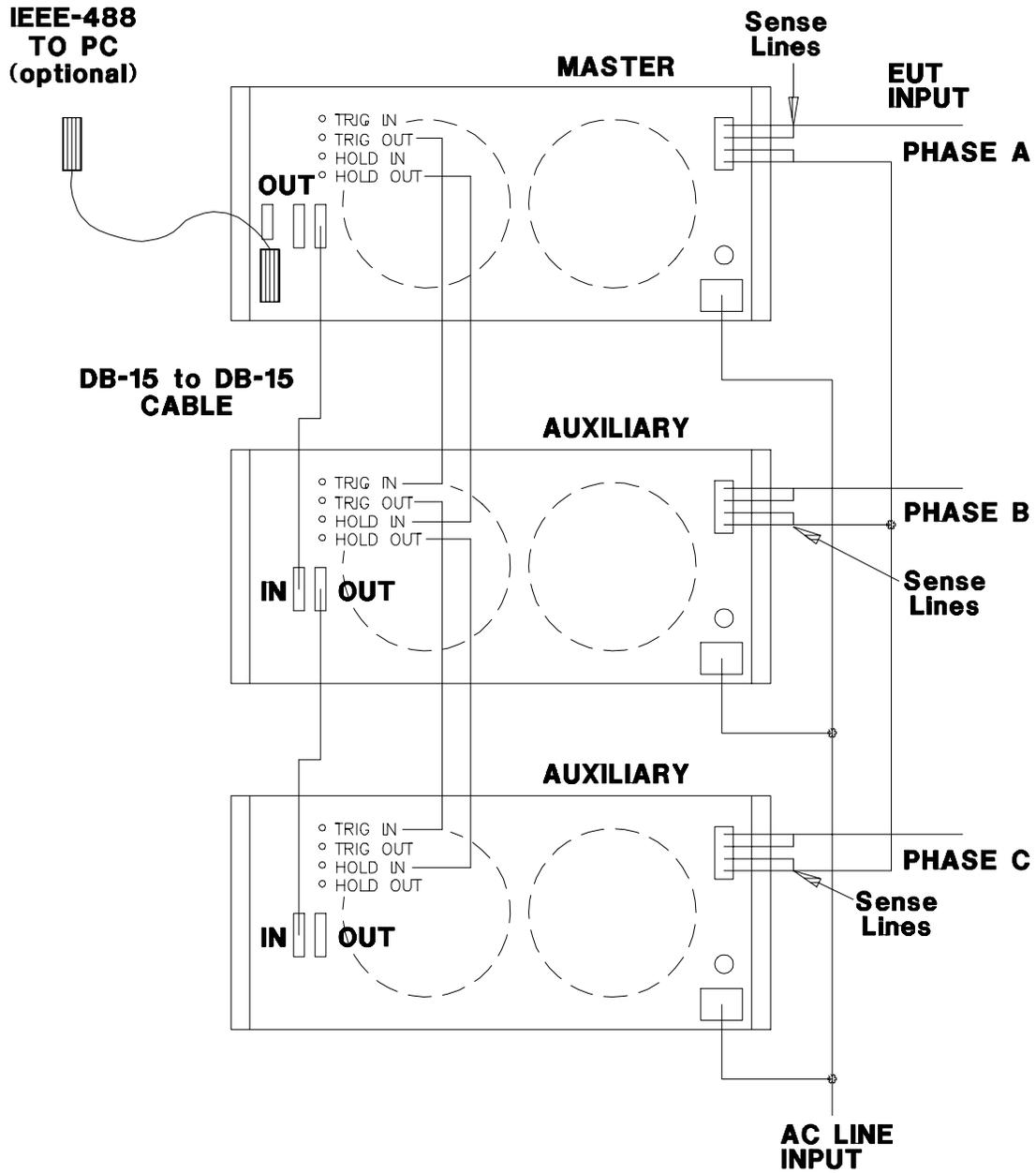
Figure 3-4: 9093LD Three-Phase DELTA Wiring
