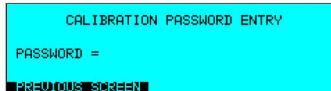
To unlock the calibration mode, the correct password needs to be entered. For the 3091LD AC load, the calibration password is: "3091". Enter "3091" without the quotes while the cursor is on the PASSWORD = field using the decimal keypad and press the ENTER key. This will bring up the actual CALIBRATION menu.
