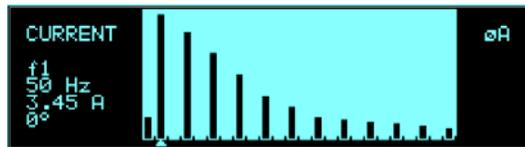
BAR mode: displays the first 50 harmonics in a graphical bar chart display.
