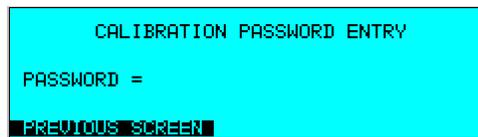
In the Password field, type 3091 using the numeric keypad and press the ENTER key to access the CALIBRATION adjustment screen. For multi phase systems, each phase needs to be calibrated in turn. Use the PHASE key on the front panel to select the phase to be calibrated for a 9093LD AC load system with one controller.
