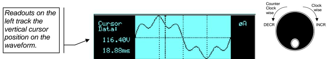
The left portion of the LCD display is used to read out the data under the vertical cursor. This cursor is a vertical dotted line that can be moved horizontally using the shuttle. As the cursor is moved, the data under the cursor is read out on the left hand side of the LCD display.
