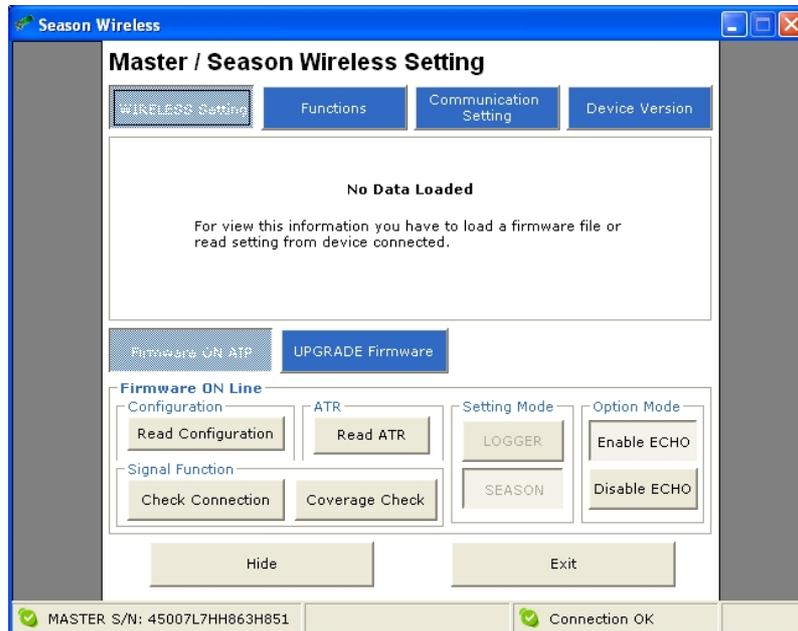
Click **Read Configuration** to display the initial settings of the device. The settings are displayed only if both components are powered and if the two antennas are correctly inserted in their respective slots.
