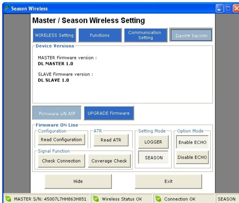
Click **Read ATR** to quickly display only the ATR that has to be sent to the remote device.
