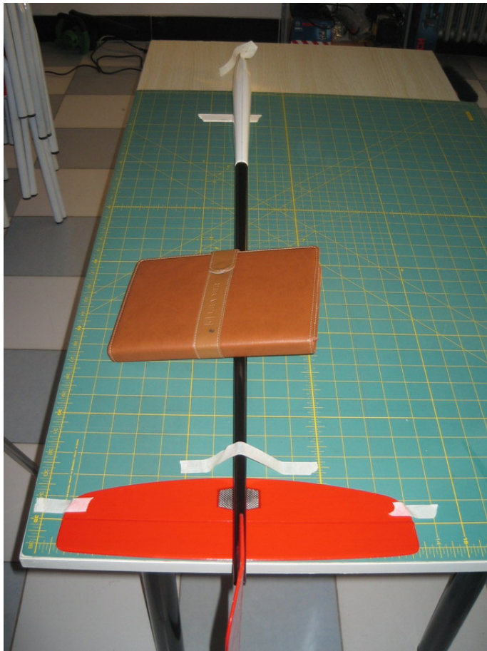
1.23. Bond the stabilizer mount and the tail boom with fast glue.
