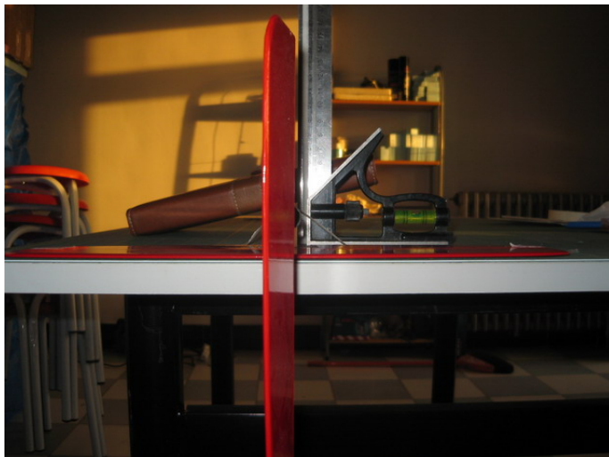
1.22. With the scale mark, adjust the stabilizer and the mount. When the stabilizer is flat on the desk, the hinge of the elevator is vertical to the tail boom.
