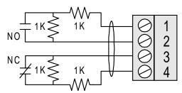
Additional inputs TMP and PFL are typically used for monitoring cabinet tamper and power failure respectively. These two inputs are not supervised and are not accessible when the board is rack mounted. These inputs are used when this board is mounted remotely mounted and cannot take advantage of the tamper and power fail detect inputs on the controller board. If these inputs are not used, install a short piece of wire at the input to indicate safe condition.
