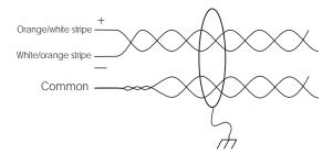
Note: For N-485 Communication Connections, twist the blue pair together and use as the common; use the orange pair as your data pair, observing polarity. Connect the external drain shield to the appropriate earth ground on one end.
