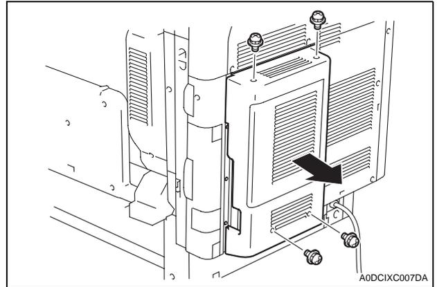
3. Remove the shield cover (two screws).
