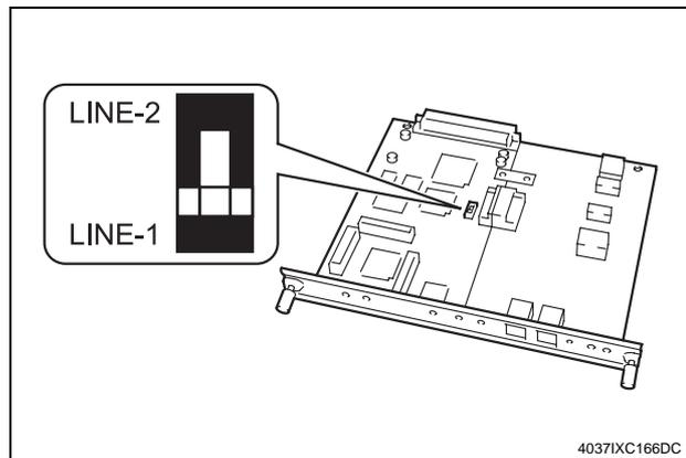
4. Insert the FAX kit and tighten the two shoulder screws.
