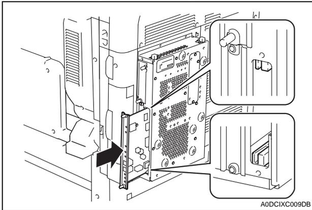
6. Reinstall the shield box cover that has been removed in step 2 (four screws).
