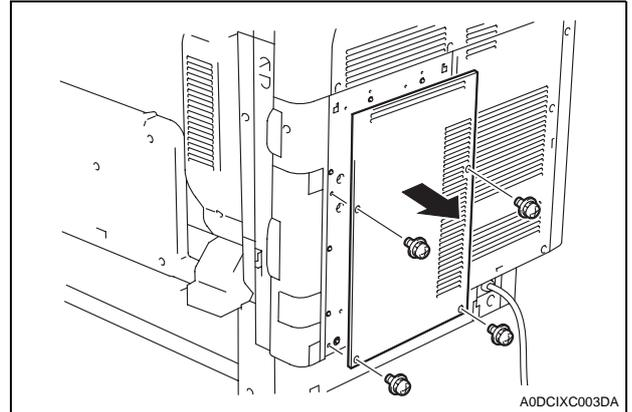
3. Remove the metal blanking plate (six screws).
