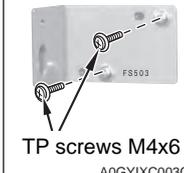
3. Remove the rear cover of the FS-521. (5 screws)
