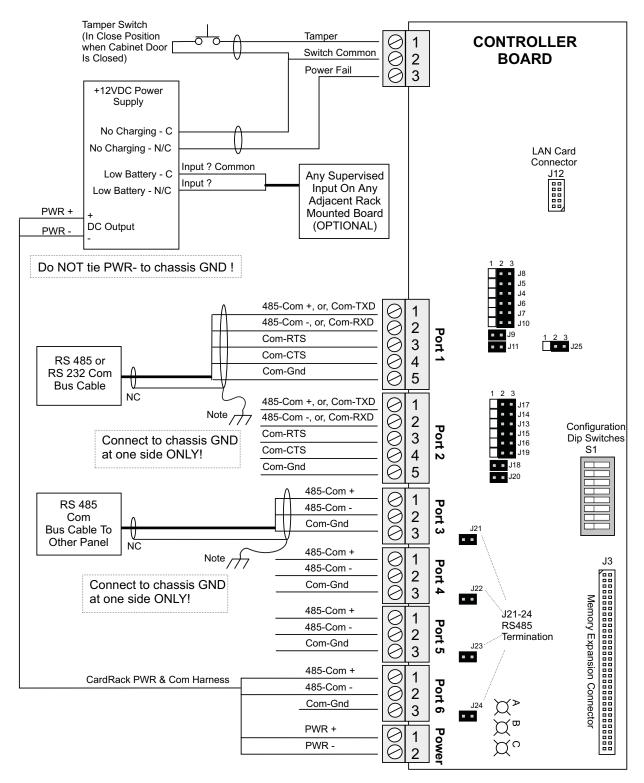
Note: For N-485 Communication Connections, twist the blue pair together and use as the common; use the orange pair as your data pair, observing polarity. Connect the external drain shield to the appropriate earth ground on one end.
