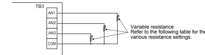
Do not apply voltage or current to AN1, AN2, AN3, or COM.
