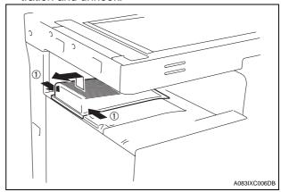
3. Remove the fixing leg and fixing leg cover of the front left leg only when the paper feed cabinet or the desk is mounted.
