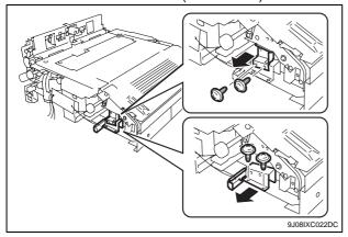
11. Remove the fixing bracket on the right side of the finisher unit (two screws).
