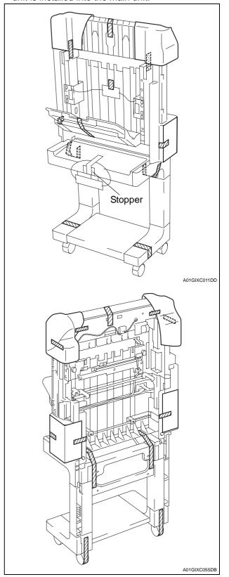
3. Remove the fixing bracket of the tray unit (three screws each).
