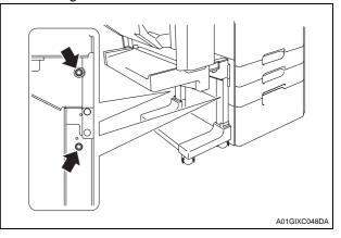
35. Reinstall the covers that have been removed in step 33 (two covers).
