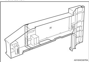
5. Remove three fixing brackets on the left side of the finisher unit (two screws).
