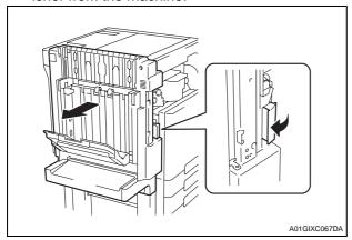
18. Connect the three connectors and a ground wire (one screw C furnished with the finisher).
