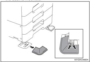
4. Peel seals off the machine (two seals).
