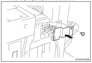
20. Install the secondary cover (two screw C's furnished with the finisher).
