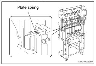
2. Remove protective tape from different parts of the tray unit.
