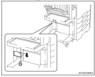
16. Attach the stopper which was removed in step 15 to the position shown in the illustration.
