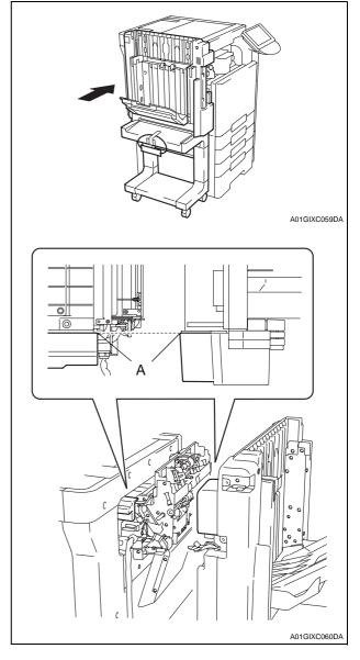
10. Fix the tray unit to the machine (four screw A's furnished with the finisher).
