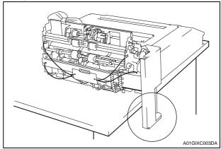
1. Remove the protective sheet and tape from the finisher unit.
