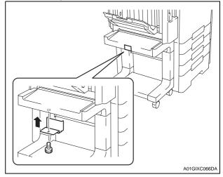
17. Pull the lock release lever and remove the finisher from the machine.
