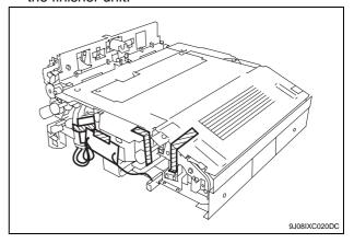
8. Remove two screws at the bottom of the finisher unit, and remove the fixing bracket.
