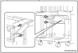
11. Install the mounting bracket B (two screw B's furnished with the finisher).
