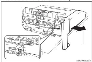
3. Remove the fixing bracket of the front cover (one screw).
