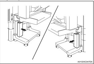
34. Loosen the two screws (left and right) shown in the illustration and make the height adjustment. Then tighten the screws.
