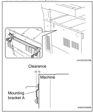
6. When the punch kit and the saddle stitcher are to be mounted along with the finisher, mount the punch kit and the creasing unit for the saddle stitcher to the finisher.
