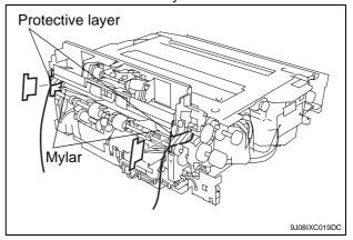
7. Remove the protective tape on the front side of the finisher unit.
