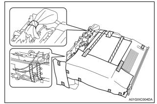
2. Remove the front cover (two screws).
