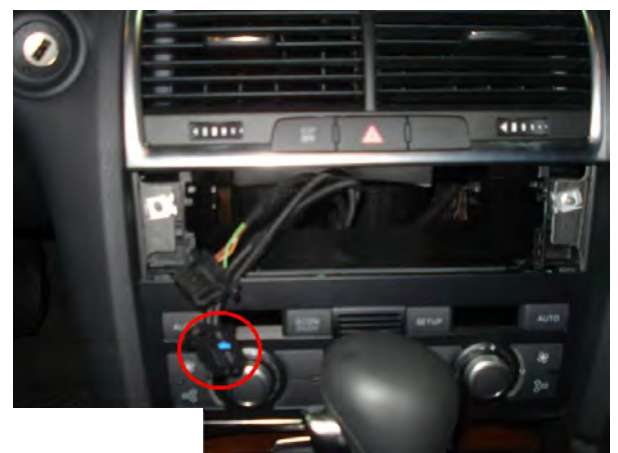
Step 3 : Change the MOST connector (indicated with red circle)
