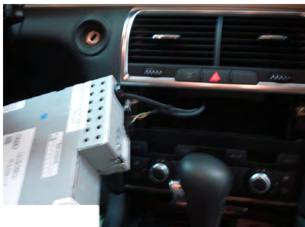
Step 2 : Disconnect the cables
