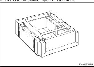
4. If the cover is installed to the position shown in the illustration, remove it (one screw).
