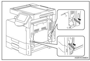
6. Holding onto the transportation handles at the right and left of the machine, place the machine onto the desk. When placing the machine, use the positioning pin in the rear of the desk to align the machine correctly with the desk.
