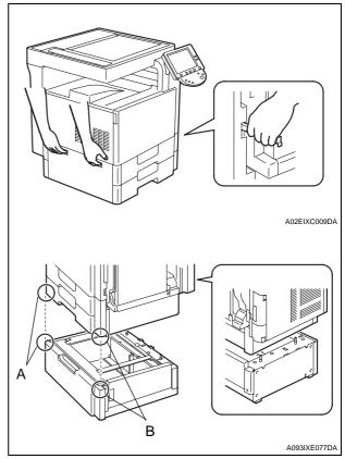
7. Secure the desk to the machine by the fixing bracket A (left) and the fixing bracket C (right). Fixing bracket A:
