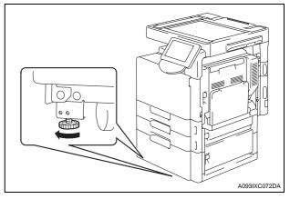
12. Install the Fixing Legs at two locations in the front shown in the illustration (six screw C's furnished with the desk).
