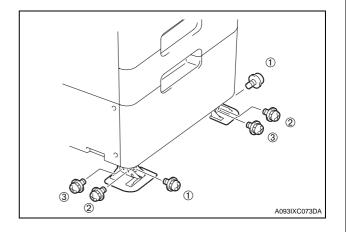
13. Install the fixing leg covers (two pieces) at two locations in the front shown in the illustration.
