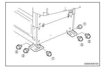
15. Install the fixing leg covers (two pieces) at two locations in the rear shown in the illustration.
