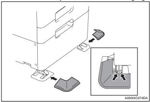
14. Install the fixing legs at two locations in the rear shown in the illustration (six screw C's furnished with the desk).
