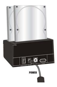
b. Once the Bays indicators are on, that means DA-70544 is ready for clone.
