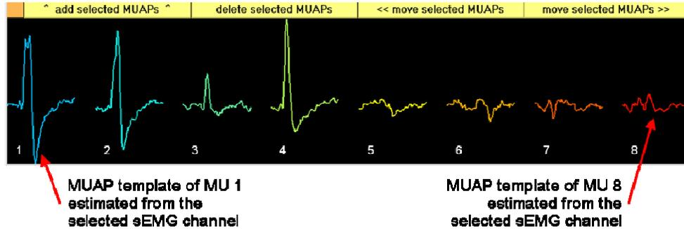
**Figure 22:** The central panel of “sEMG editor” window with MUAP templates. MUAP templates are estimated by spike triggered averaging of the selected sEMG channel.
