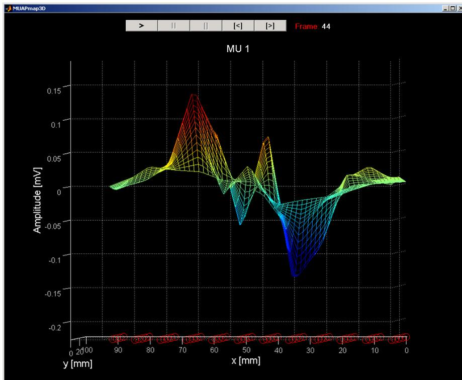
**Figure 40:** 3D rotation of the axes; the axes of the 3D plot can be freely rotated by clicking on the axes and dragging the cursor in the direction you want to rotate the plot.
