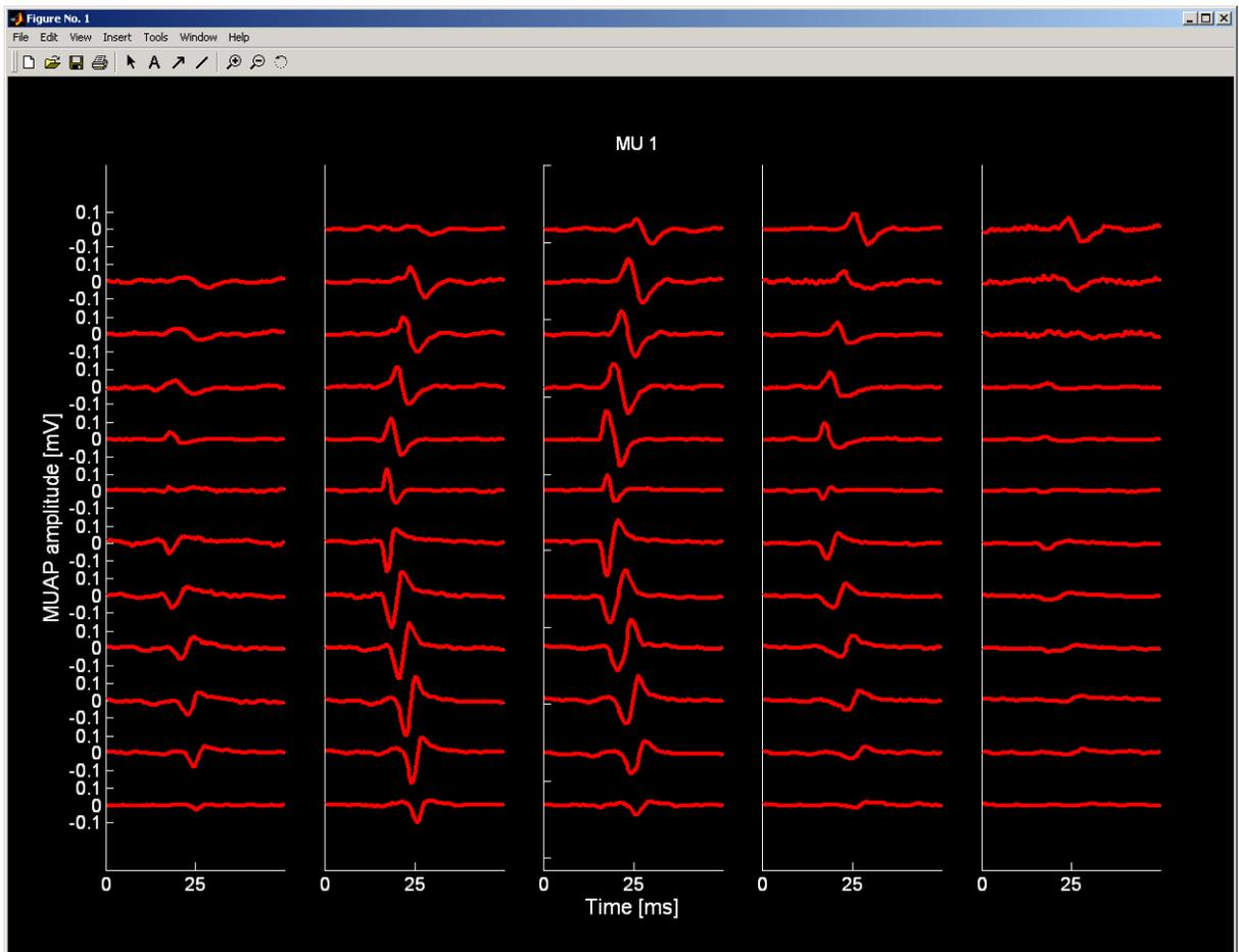
Figure 35: Multi-channel MUAPs estimated by spike-triggered averaging of sEMG signals. sEMG signals were recorded with a grid of 61 electrodes arranged in 5 columns and 13 rows. The location of the innervation zone, tendon regions and propagation of motor unit action potentials are visible.
