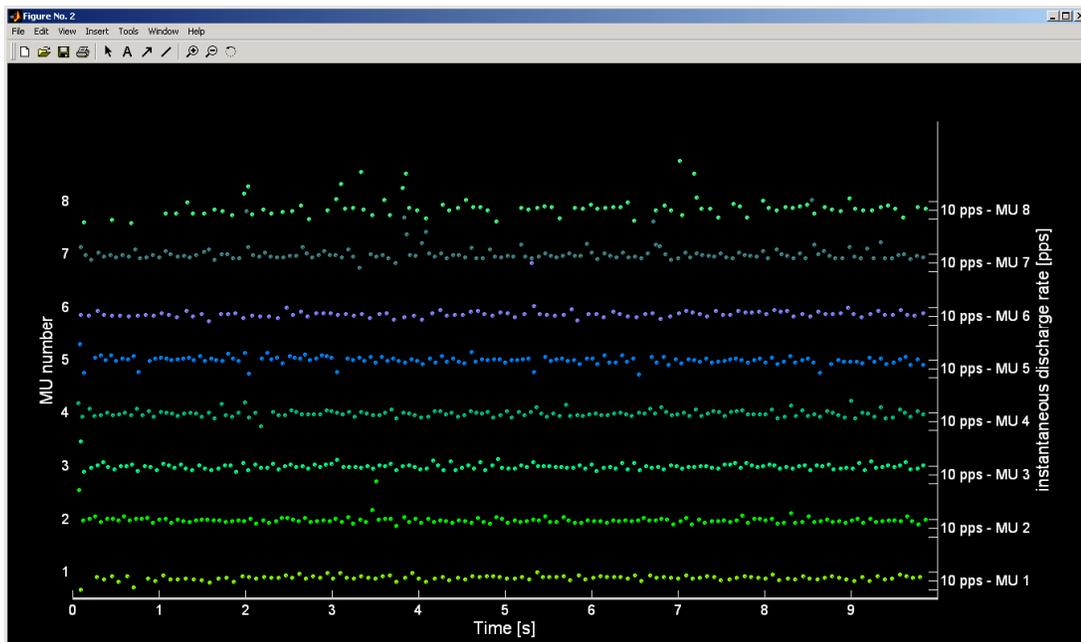
Figure 31: Plots of reconstructed MU discharge patterns. Vertical axis on the left displays MU IDs, vertical axis on the right displays the instantaneous discharge rates (in pulses per second - pps). The tick lines on the right denote the discharge rates of 5, 10 and 15 pps, respectively. Discharge patterns of different MUs are depicted one above the other.
