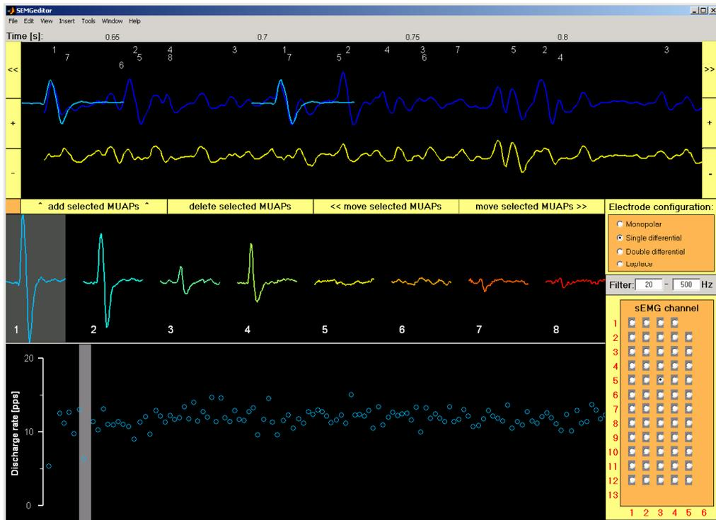
**Figure 24:** MU 1 is selected by clicking on its MUAP template in the central panel. MUAP occurrences and instantaneous discharge rates of selected MU are automatically depicted in the top and the bottom panel, respectively.
