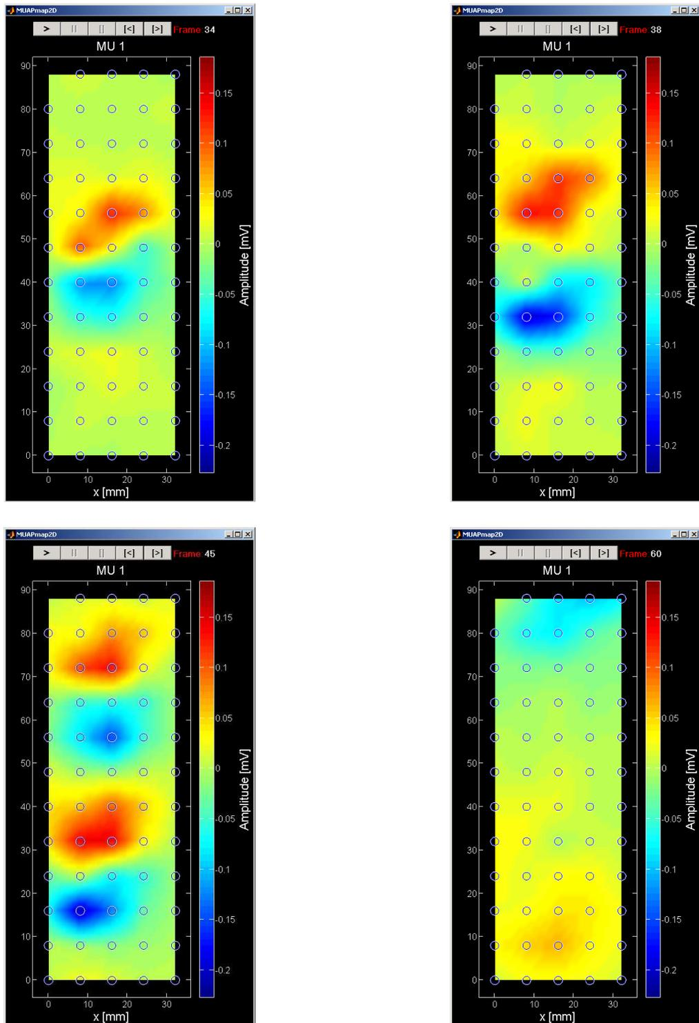
**Figure 37:** Pseudocolor animation of a MUAP generation, propagation and attenuation process. MUAP amplitudes on different sEMG channels (black&white circles) specify the colours of corresponding points on the 2D map. Colours of intermediate map points are calculated by the bilinear interpolation of the MUAP amplitudes in four adjacent sEMG channels.
