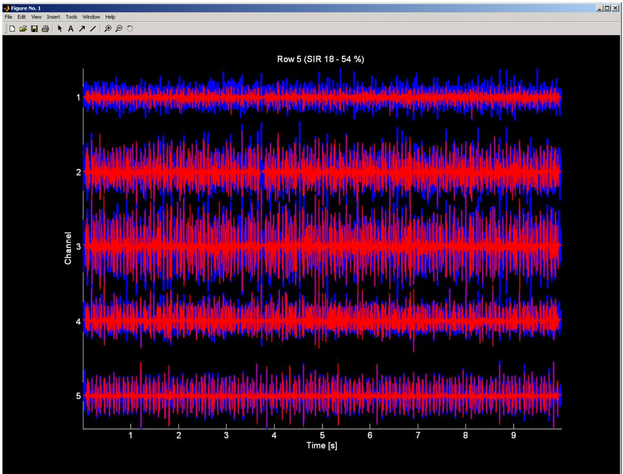
**Figure 42:** Matlab figure of selected sEMG channels and corresponding reconstructed MUAP trains. The range of SIRs of the depicted channels is displayed on the top of the figure.
