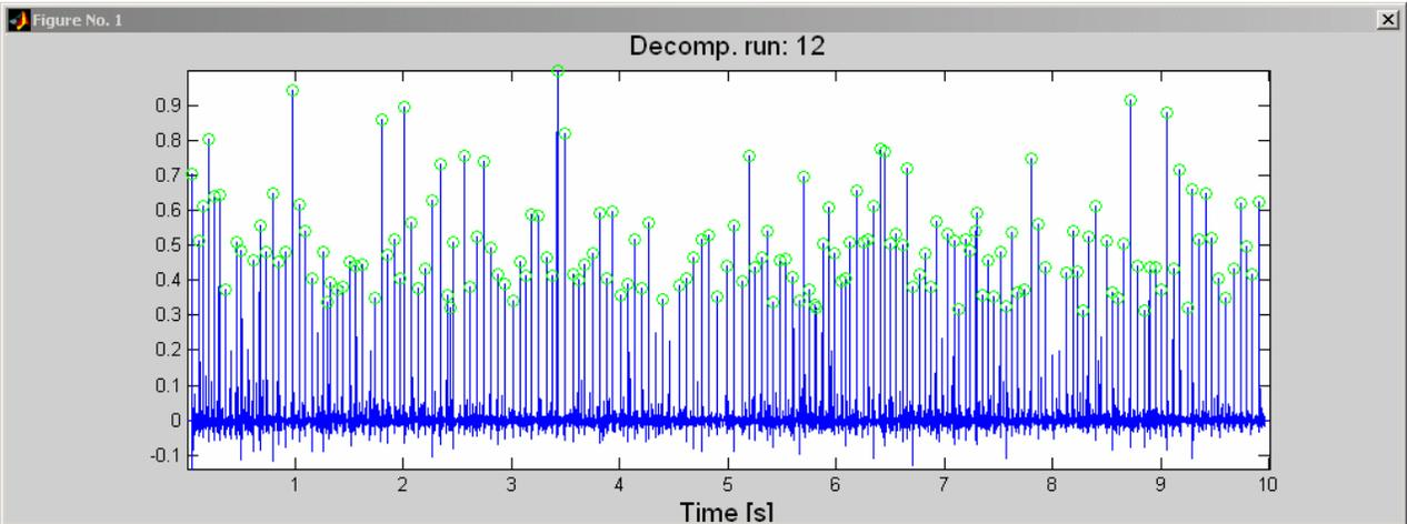
**Figure 15:** MU discharge pattern, reconstructed in the 12<sup>th</sup> iteration of the gCKC decomposition technique. Each pulse corresponds to a single MU discharge. Average discharge rate and coefficient of variability of inter-pulse interval are within the expected range of values. Thus, the selected MU discharges are depicted by green circles.
