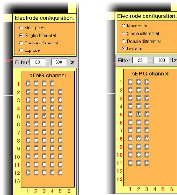
**Figure 29:** Command frame of “sEMG editor” with “sEMG channel” panel, Butterworth band-pass filter cut-off frequencies and “Electrode configuration” panel for single differential electrode configuration (*right*) and Laplacian electrode configuration (*left*).
