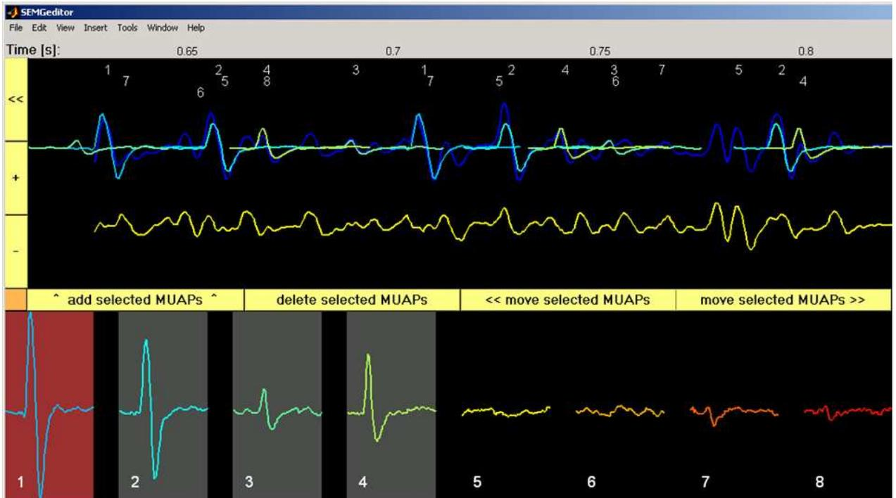
**Figure 26:** Double click on a MUAP template of MU 1, followed by a click on a “add selected MUAP” button adds the MUAP to the top panel. The MUAP template selected by double-click is depicted by a red rectangle.
