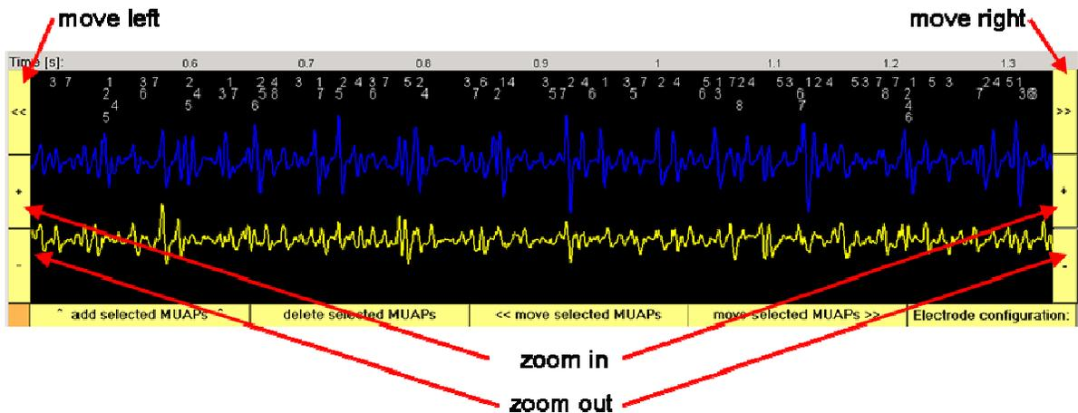
**Figure 21:** The top panel of “sEMG editor” window with buttons for moving left/right and zooming in/out on displayed signals.
