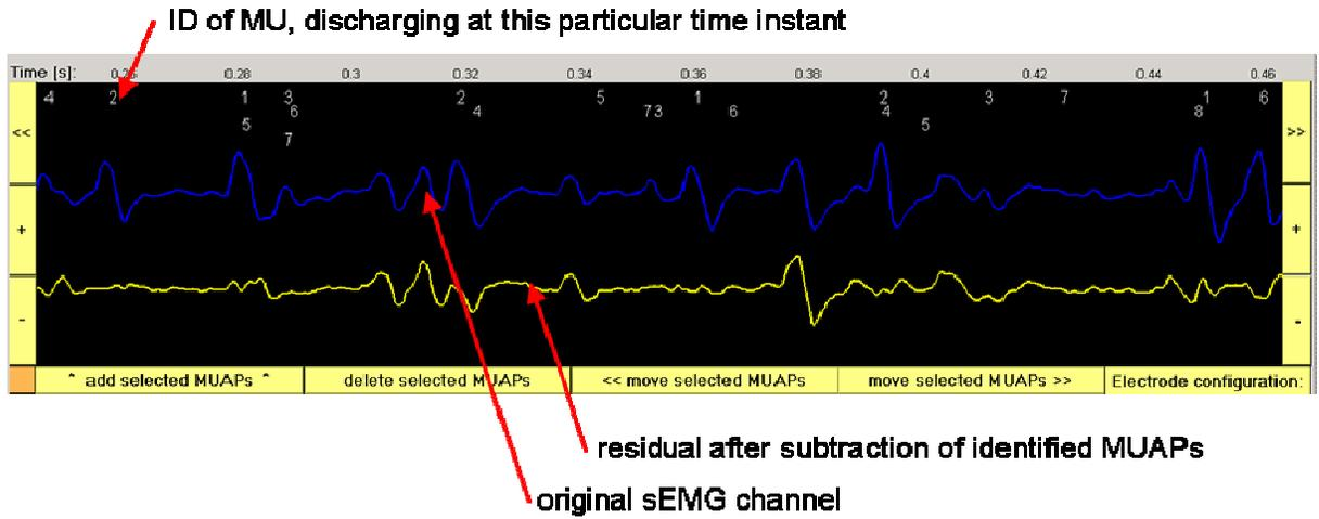
**Figure 20:** The top panel of “sEMG editor” window with original sEMG channel (blue line) and residual after subtraction of the identified MUAPs (yellow line)
