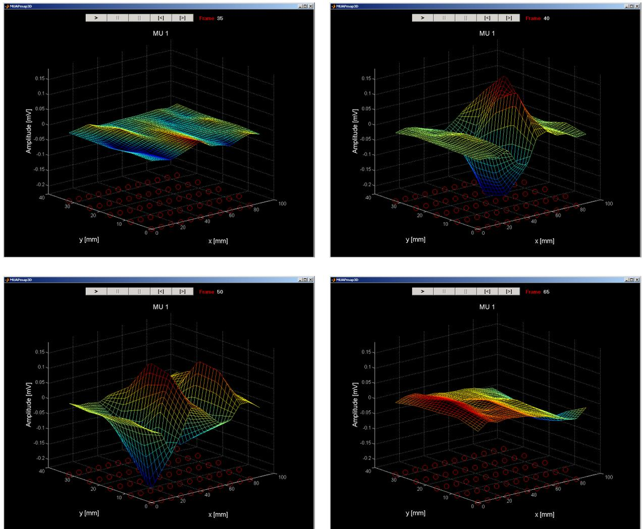
**Figure 39:** 3D animation of MUAP generation, propagation and attenuation. MUAP amplitudes on different sEMG channels (red circles) specify the height of corresponding points on a 2D map (heights of intermediate map points are calculated by the bilinear interpolation of the MUAP amplitudes in four adjacent sEMG channels).
