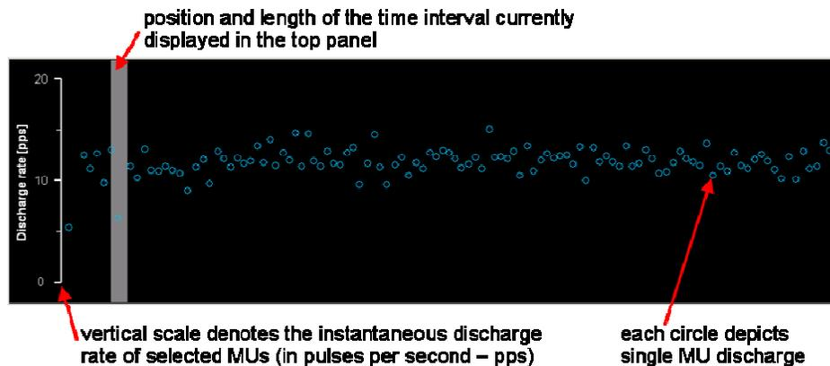
**Figure 23:** Bottom panel of the “sEMG editor” window with the instantaneous discharge rate plot of a selected MUs.
