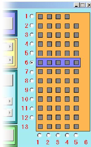
**Figure 5:** Channel selection frame; the number of acquired channels and their relative spatial organization is displayed (grey rectangles). Red numbers at the left hand site and at the bottom denote the corresponding rows and columns of electrodes, respectively.
