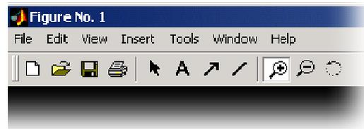
**Figure 9:** Matlab figure toolbar with tools for zooming in/out on a figure, and for saving and printing the figure.
