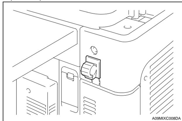
6. Run the authentication unit cable through the hole in the working table.
