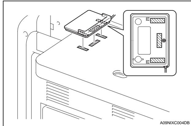
5. Attach the cord clamp onto the position shown in the illustration.
