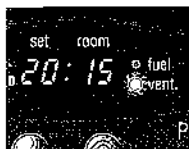
J: A blinking VENT indicator light is a sign that you need extra ventilation.
