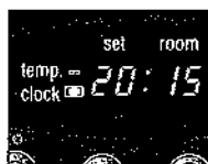
E: When the CLOCK indicator light stops blinking, the setting has been locked to the indicated value.
