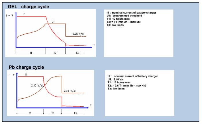
Fig.3: Charge curves available on EDM
