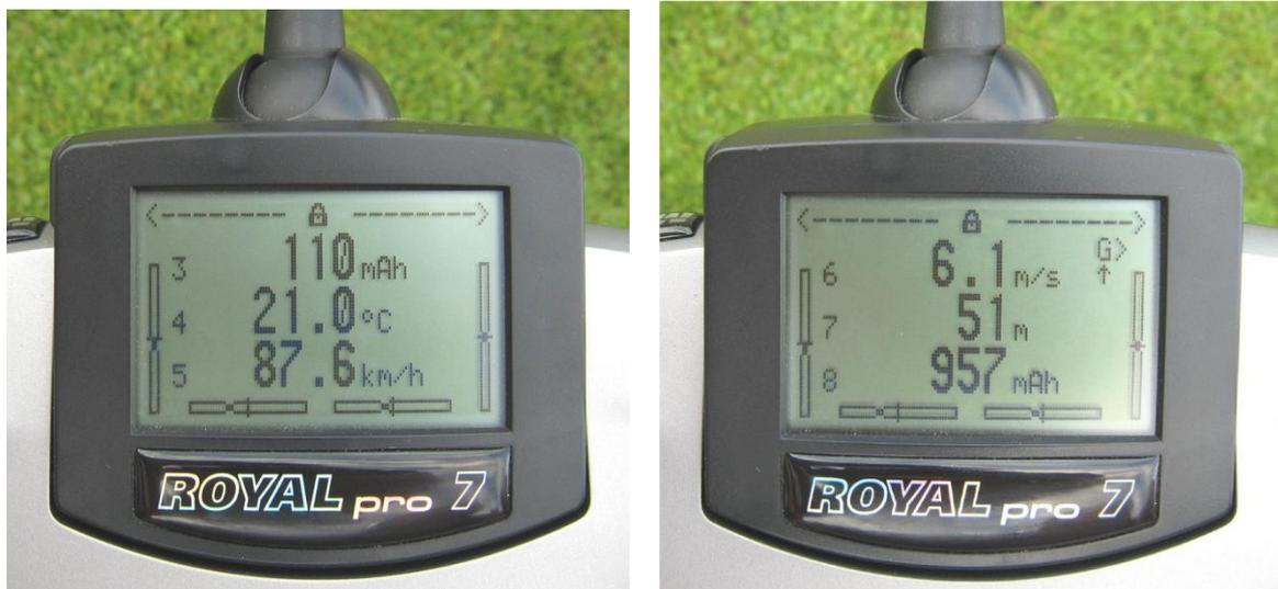
The settings for telemetry can be made either with the UniDisplay ( see chapter 7) or with our “SM GPS-Konverter” software on a PC.
