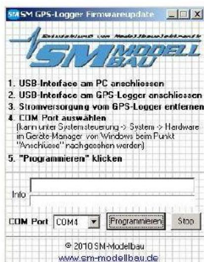
With our USB interface a firmware update can also be uploaded to the GPS-Logger. To make an update, a Windows PC with USB interface and installed driver for the USB interface is necessary.
