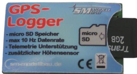
The card is inserted into the slot on the back and pushed in until it clicks and is flush. The GPS-Logger does not have an ejector for the memory card, the card is simply pulled out again with the fingers.
