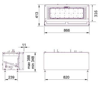
ATTENTION: an installation hatch must also be installed of 20cm \* 20cm\* 20cm (height \* width \* depth) containing the gas control valve and the receiver. Ensure that there is adequate space around the appliance to be able to install this installation hatch.
