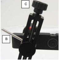
Once the vertical balance is set, tighten the position lock lever (B) and set the tensioner knob to your preferred level of resistance. You should be able to tilt effortlessly and the tilt mechanism should hold any angle unaided.
