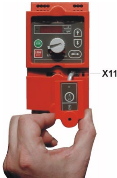
Fig. 2: Connection to MOVITRAC® 07
