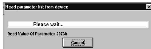
Figure 52: The CMD tool reads device parameters, i.e. PCP communication is OK.
