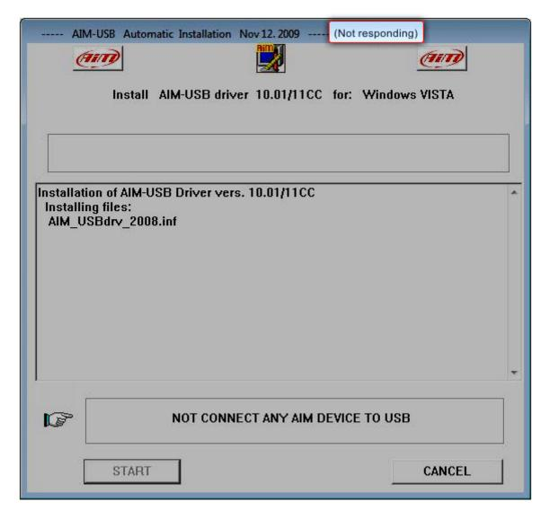
The program is busy installing AIM USB Driver. Microsoft Windows signals this adding "Not responding" to the mask title of "AIM-USB Automatic Installation" window. Just wait for a few seconds and the window will become active again. AIM is working to avoid this situation.
