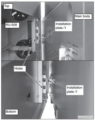
9. Fix the RU-509 and the installation plates /3 with the screws. (TP screw M4x8: 2)
