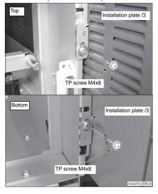
10.Plug in the RU-509 power cord and fix it in the clamp. (Sems II screw M4x8 : 1)
