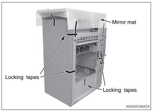
3. Open the front door and remove the locking tapes and the bundled item.
