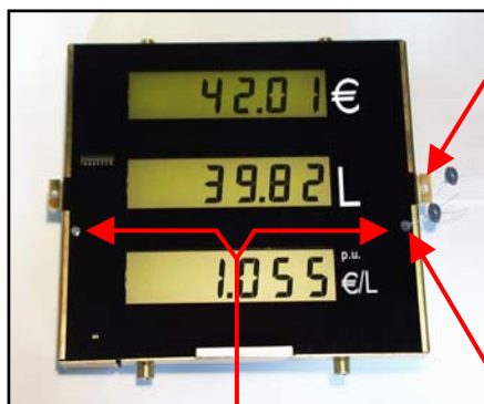
Photo 11: Display of computing head TW1-B e TW1nA-B front view
