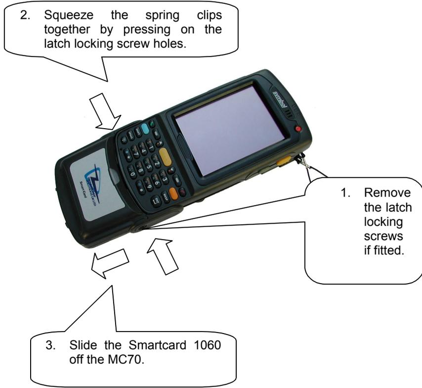
**Figure 3: Detaching from an MC70**
