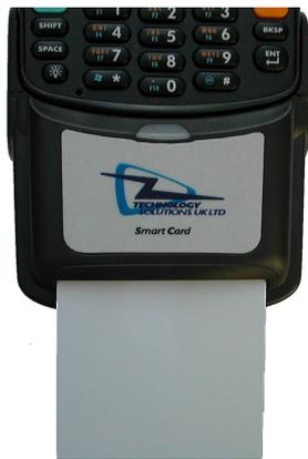
Correct orientation; the smartcard contacts are facing downwards.
