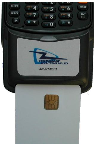
Incorrect orientation; the smartcard contacts are facing upwards.
