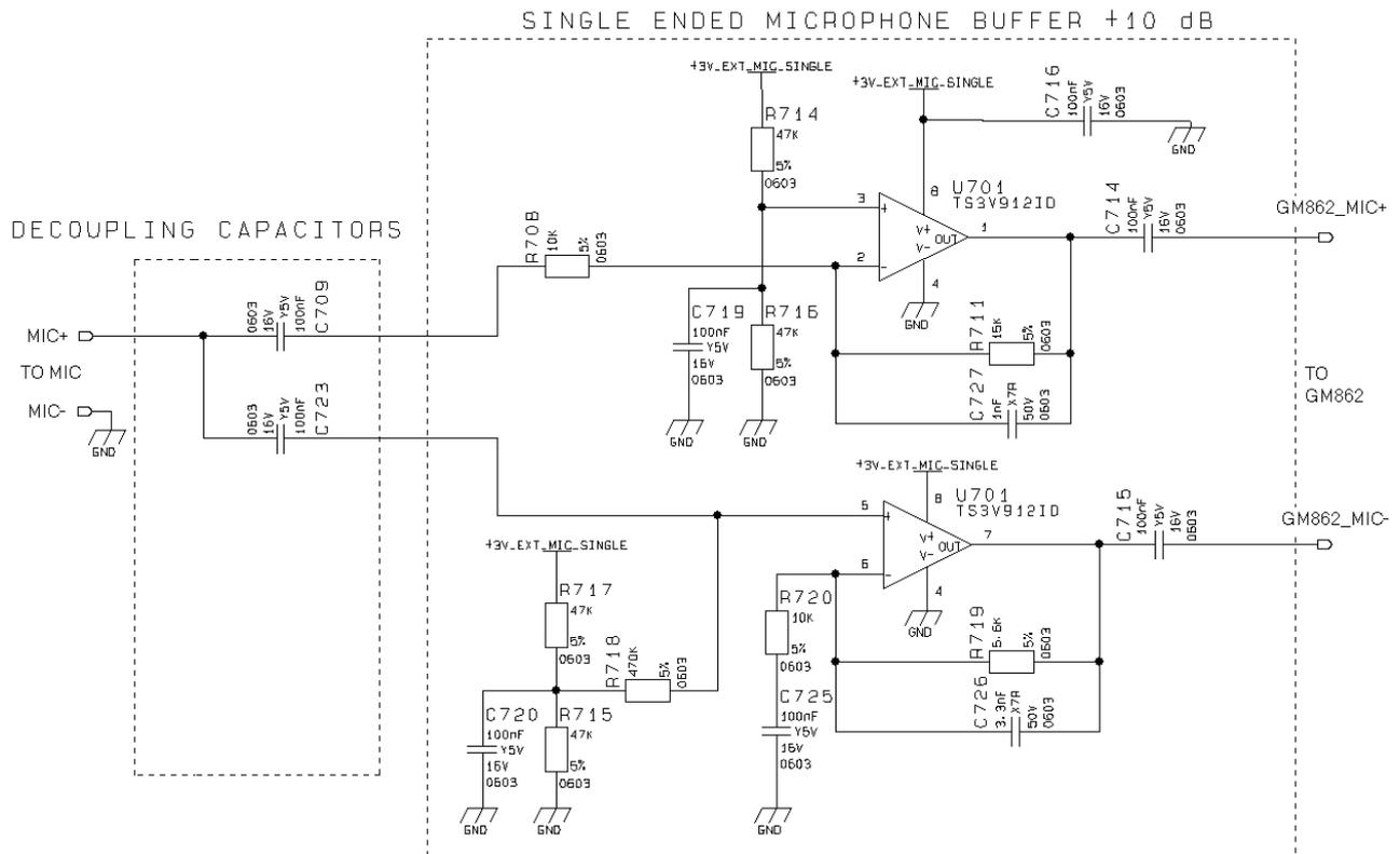
The schematic does not include the required mic. biasing circuitry. For the biasing the same circuit as seen before can be used; to be noticed that the capacitor C3 on the unbalanced biasing circuit is not anymore needed if this Buffered design is used.
