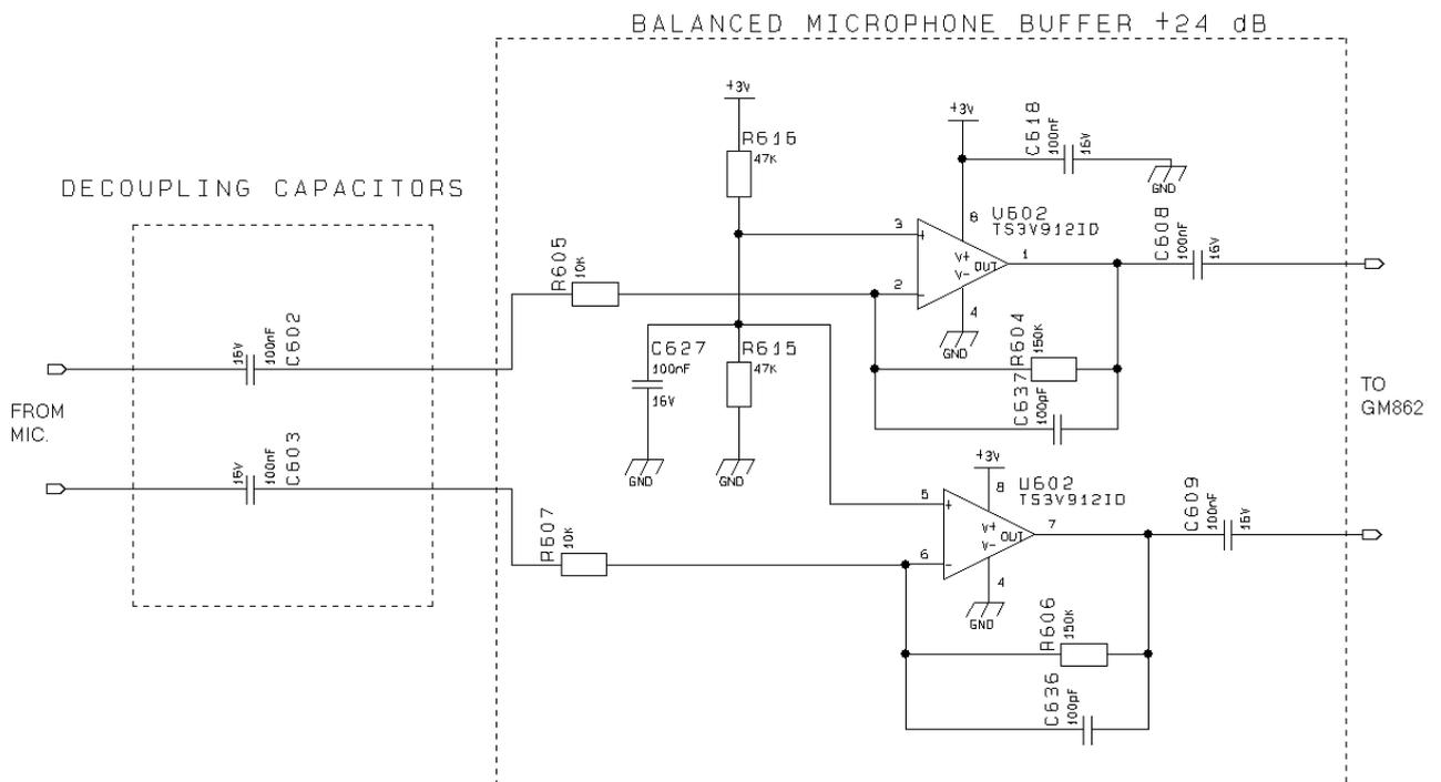
This circuit has a gain of 15 times (+24 dB), and is therefore suited for the internal mic. input, having a microphone with a sensitivity close to the suggested one (-45 dB<sub>Vrms/Pa</sub>), if the used microphone has a different sensitivity, or if the buffer is connected to the external mic. input, then a gain adjustment shall be done by changing resistors R604-R605 and R606-R607 and as a consequence the capacitors C636 and C637 to maintain the bandwidth 150-8000 (-3dB).
