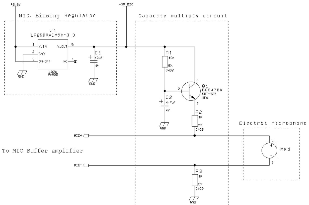
**NOTE:** In the balanced application the resistors R2 and R3 must have the same value to keep the circuit balanced.
