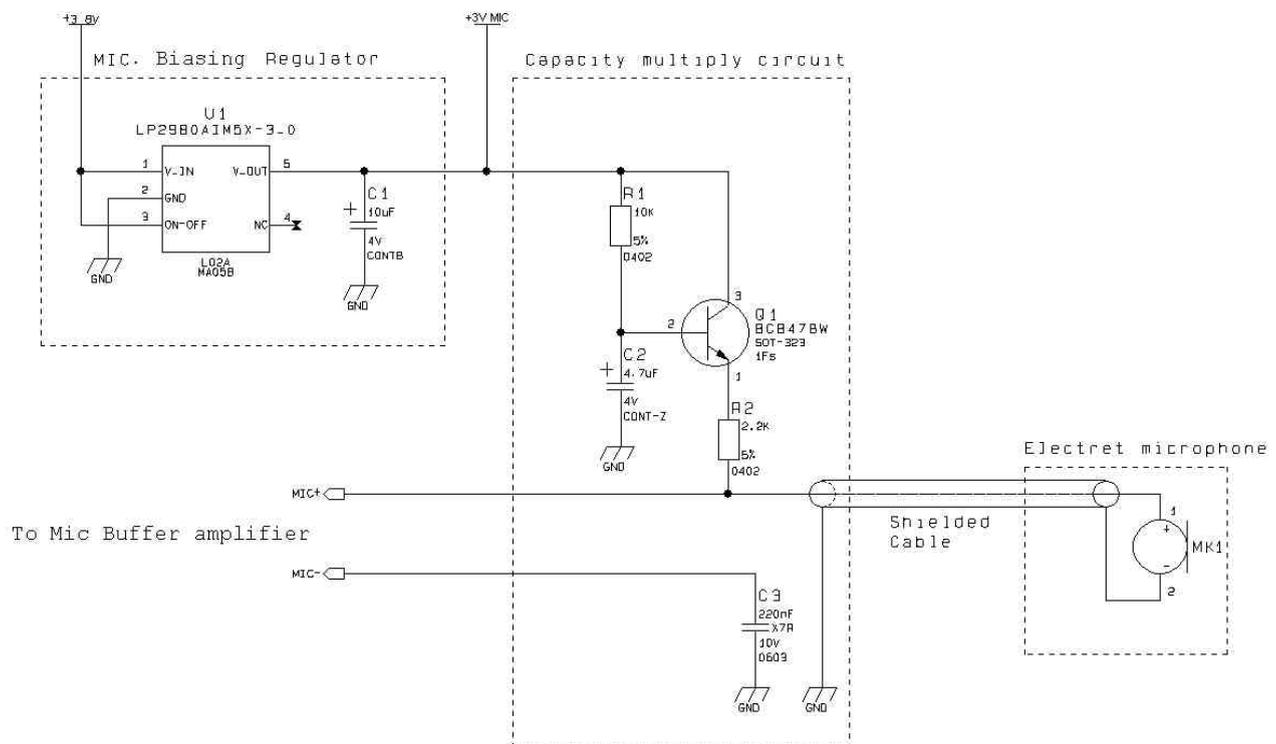
**NOTE:** In the unbalanced application the capacitor C3 shall be > 200nF otherwise the frequency response will be cut at low band frequencies (down to 300Hz). This capacitor can be placed close to the MIC- pin (EXT\_MIC- or INT\_MIC- depending on the audio path chosen) or if possible it should be placed close to the shielded cable connector. If the ground return path is well designed, then it is possible to eliminate the C3 capacitor, provided the buffer is close to the mic. input.
