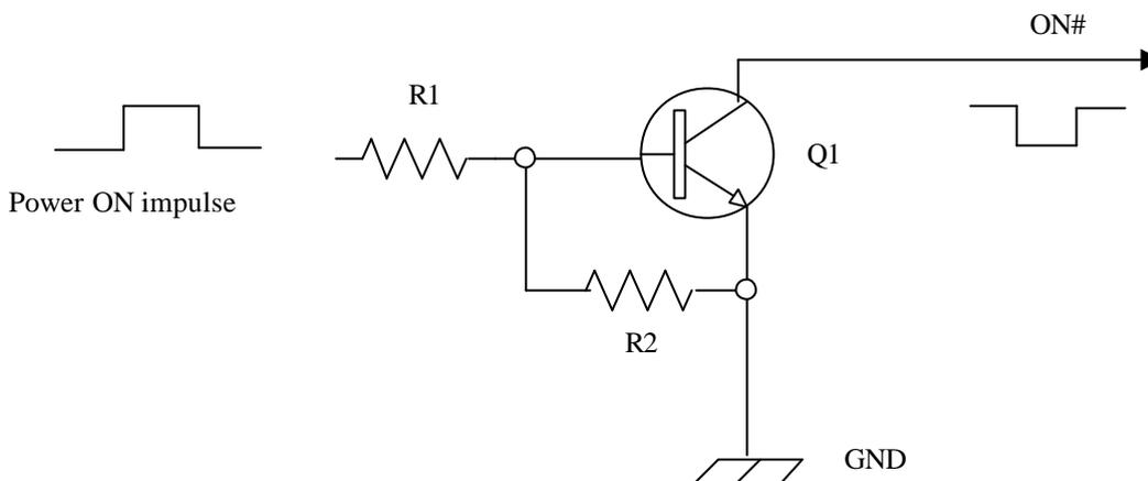
**NOTE:** don't use any pull up resistor on the ON# line, it is internally pulled up. Using pull up resistor may bring to latch up problems on the GM862-GPRS power regulator and improper power on/off of the module. The line ON# must be connected only in open collector configuration.
