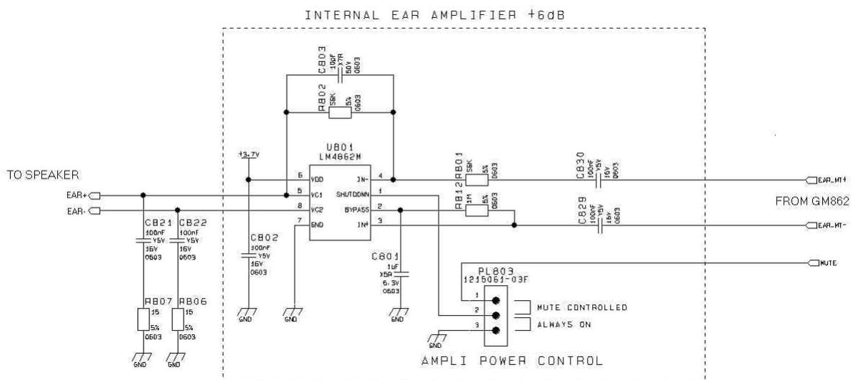
Some amplifier require a low impedance load at high frequency in order to avoid auto oscillation, this can be made with a capacitor (100nF) in series with a resistor (150).
