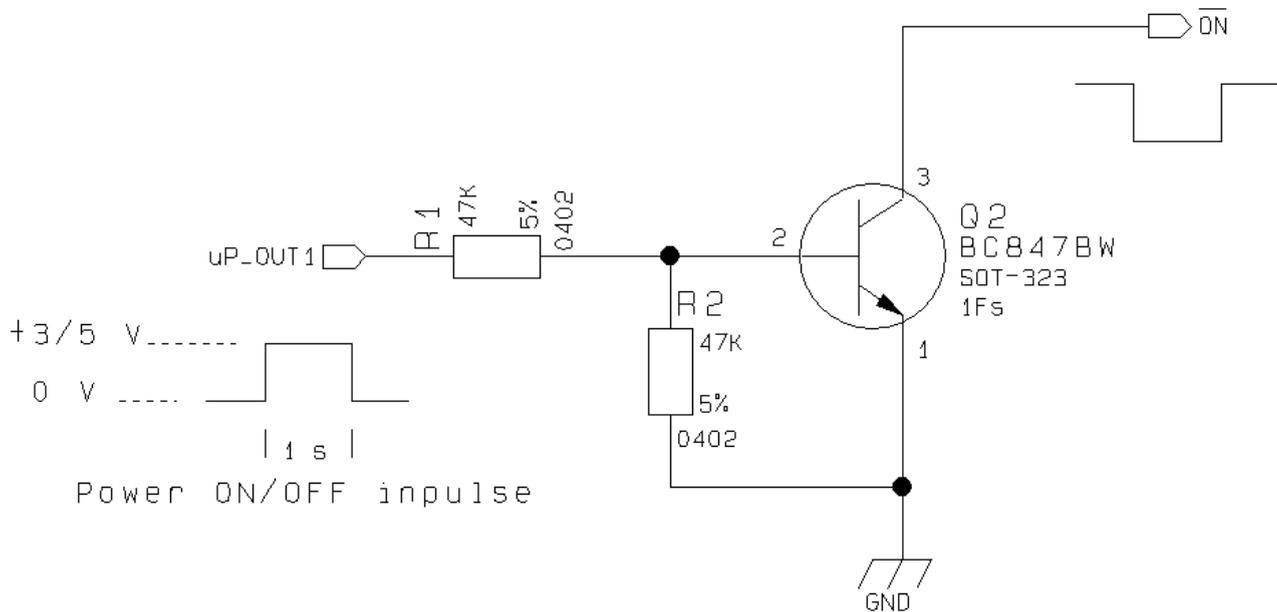
2- Let's assume you need to drive the ON# pin directly with an ON/OFF button:
