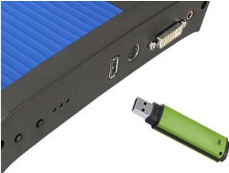
The VGADVI Broadcaster copies to the inserted USB flash drive, only files recorded before inserting the flash drive, starting from the oldest record to the newest. The
