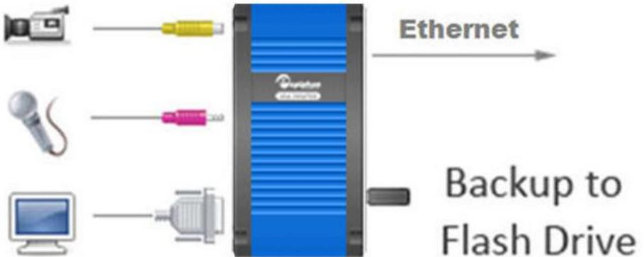
A flash drive can be connected to the VGADVI Broadcaster any time. Stick a flash drive into a USB port on the device and press lightly. The stick fits into the port only one way. After inserting, the VGADVI Broadcaster will recognize the stick, however, this occurs without any user notification whatsoever.
