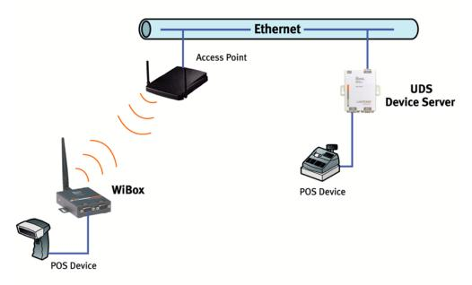
Figure 2-3. Serial Tunneling Infrastructure Example
