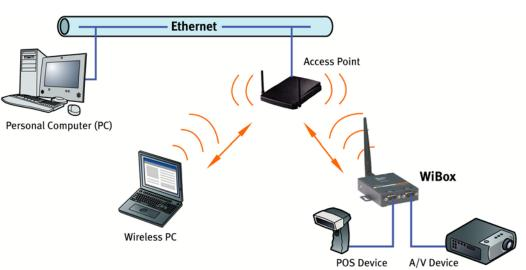
Figure 2-1. Serial Tunneling Infrastructure Network Example
