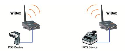
Figure 2-4. Direct WiBox to WiBox Connection
