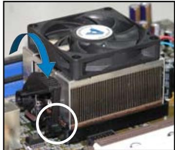
5. When the fan and heatsink assembly is in place, connect the CPU fan cable to the connector on the motherboard labeled CPU\_FAN.
