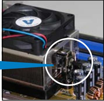
3. Align the other end of the retention bracket (near the retention bracket lock) to the retention module base. A clicking sound denotes that the retention bracket is in place.
