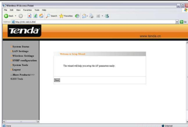
You can select “Running Status”, “LAN Settings”, “Wireless Settings”, “SNMP Settings” and “System Tools” on the left menu. Click “Next” to enter the wireless working mode setup page. W301A supports two working modes: wireless AP (AP), Bridge (WDS). Select a working mode to configure the settings. For more details please refer to the following chapters.
