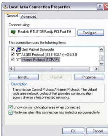
Choose the “Use the following IP address”, enter the IP address as: 192.168.0.xxx. (xxx ranges 1–253), Subnet mask is: 255.255.255.0(As Shown in Fig- 5)
