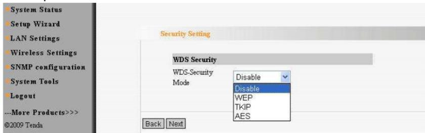
“WDS Security Setting” is used to encrypt the AP and authorize the device to establish bridge. Only when the passwords of the devices in bridge are consistent, the communication can get through normally.
