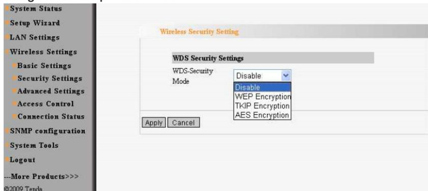
WDS security setting provides three encryption modes: WEP encryption, TKIP encryption and AES encryption.
