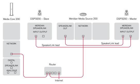
The Media Source 200 can be connected to a Meridian Audio Core product such as the AC200, or directly to a pair of DSP loudspeakers such as the DSP3200, to play music from a Meridian Digital Media System in a separate zone. The examples show the music stored on a Media Core 200.
