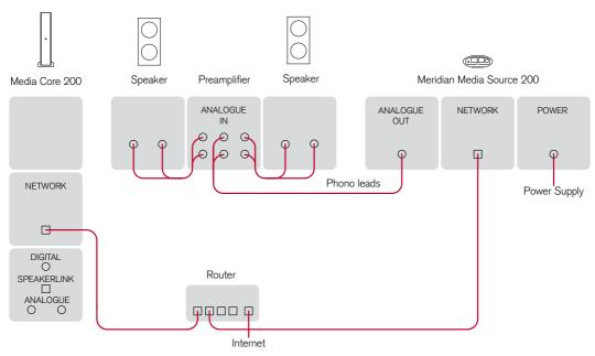
The Media Source 200 can be connected to one of the inputs on an analogue preamplifier to provide access to the music on your Meridian Digital Media System. This example shows the music stored on a Media Core 200.
