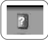
A monitor marked with a question mark indicates that an “unknown” monitor has been detected. (This icon is darker in colour than the previously mentioned ‘monitor not found’)
