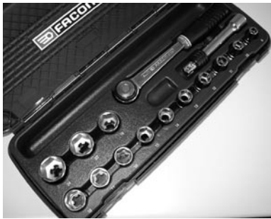
Flex ratchet and Socket wrench bits sizes 8 -19
