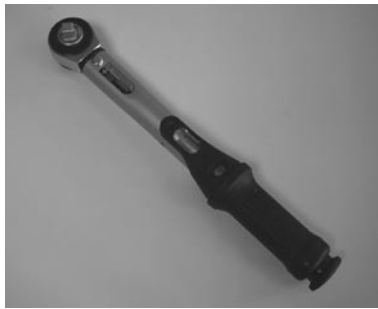
Torque wrench Measurement range 10 -25 Nm
