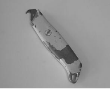
Stanley knife with sickle hooked blade and standard blade
