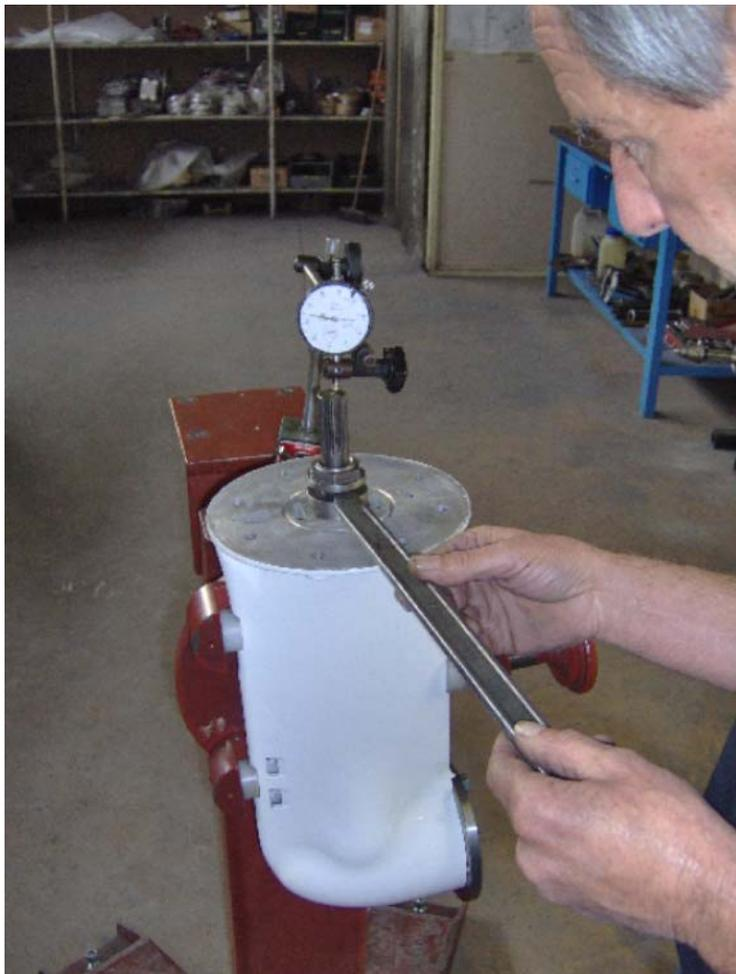
On the end of the shaft, assemble a dial gauge and detect the axial shifting as per scheme n°3.
