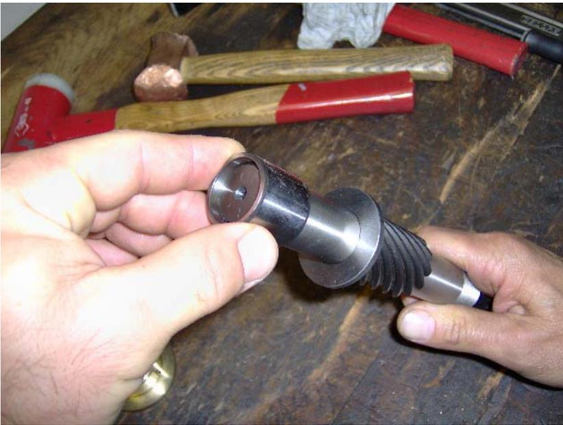
Warm the ring (ref n°5) up to 120 °C, put the ring into shaft (ref n°1) as per picture, with the help of a cylindrical stopper if necessary
