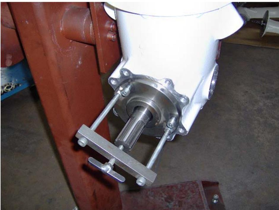
Insert the gear group previously preassembled, apply tooling (tool SP 60-03) as per the picture, on the input shaft. Screw the centre pin until the gear gets the position
