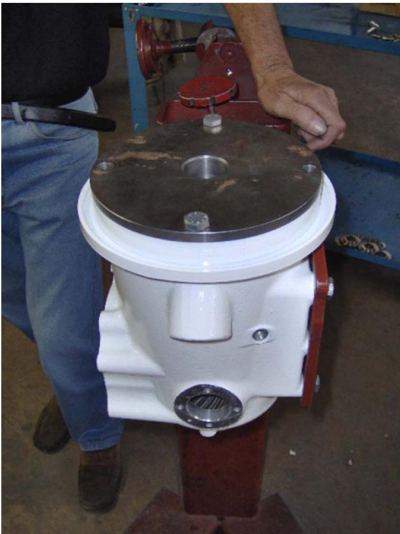
Insert the tooling (tool SP 60-02) to center the clutch group into the cover upper assy. Tighten it with the two screws.
