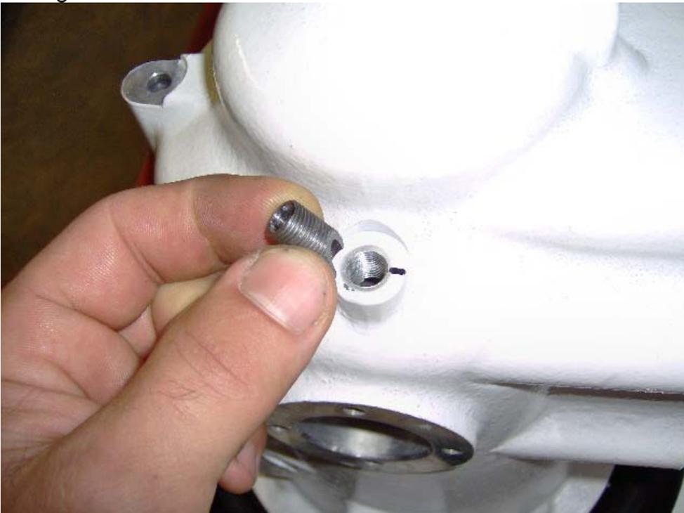
Put the fitting on the location of the breather plug, screw the fitting all the way, positioning
