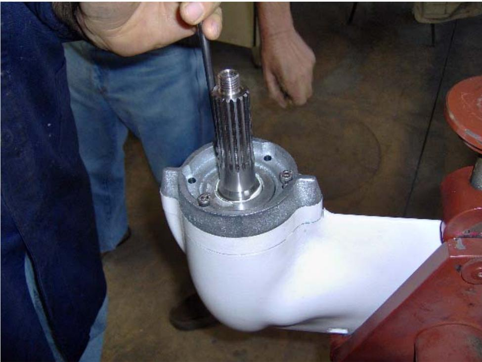
Assemble the zinc ( rif. n° 84) and tighten with screws ( rif. n° 91)
