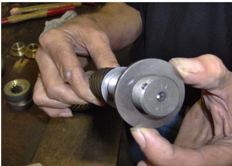
Put shim (ref. n°4) all the way down into the shaft.
