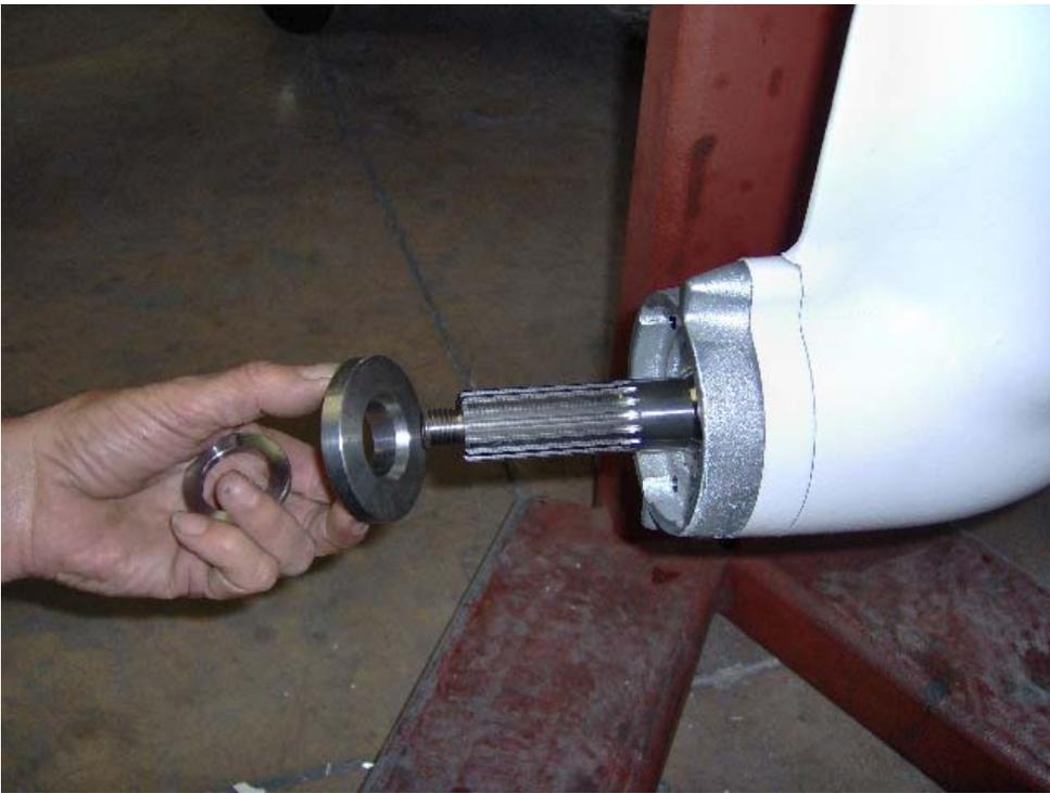
Place the spacers ( rif. n°85) on the output shaft, protecting the splined part applying a damping layer.
