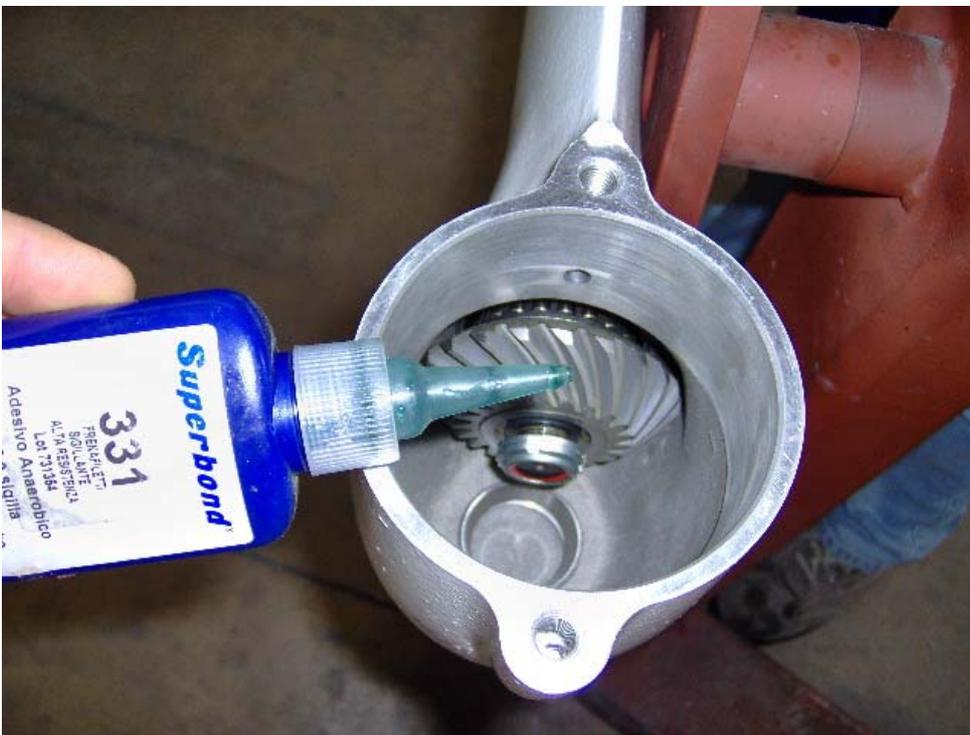
Disassemble the adjustment tooling, position the shims, reassemble the components as shown previously, when reassembling the nut ( rif. n° 70) use drops of thread locker.
