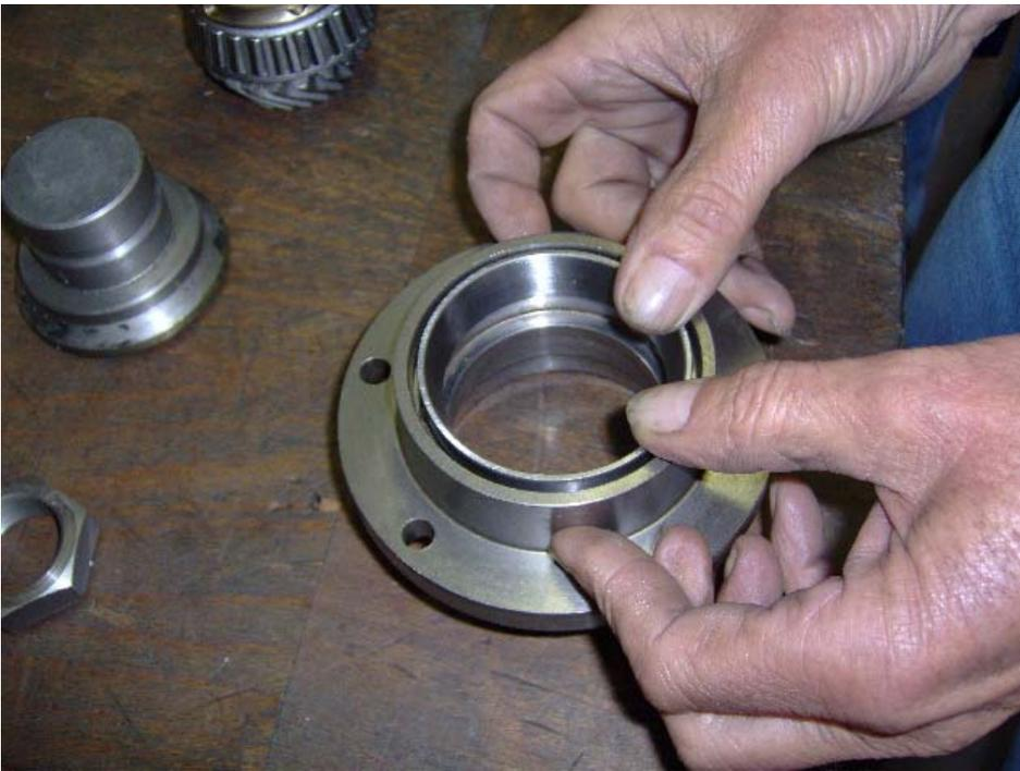
Put the bearing bowl (ref. 19 and 22) into the bearing housing (ref. n° 14) all the way down.
