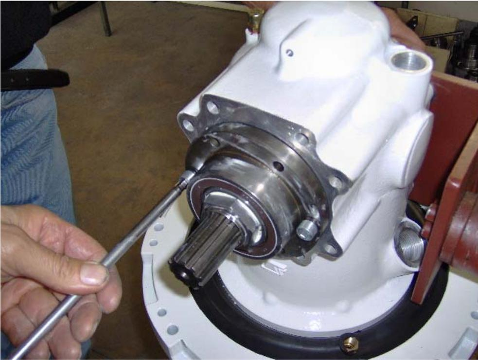
Put the gear group into the cover group, tighten the fixing screws,
