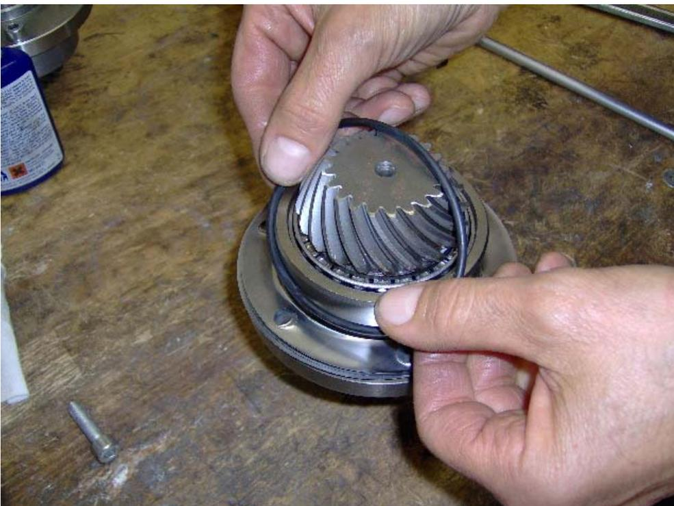
Put on as shims as to add 0.05 mm to the value detected by the thickness gauge.
