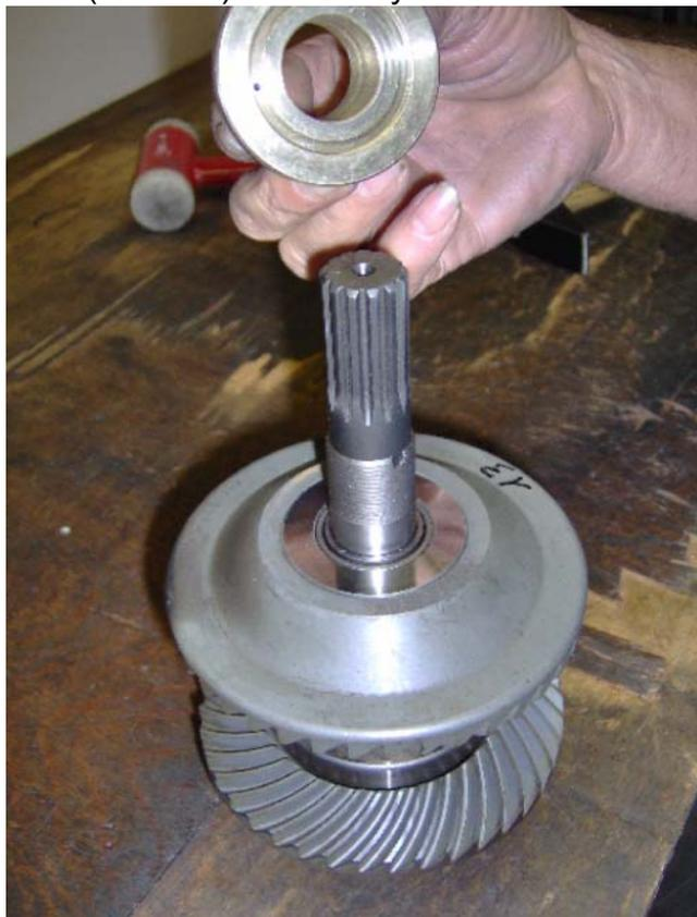
Warm up ring (ref. n°5) up to 120 °C, position it all the way down into the shaft.
