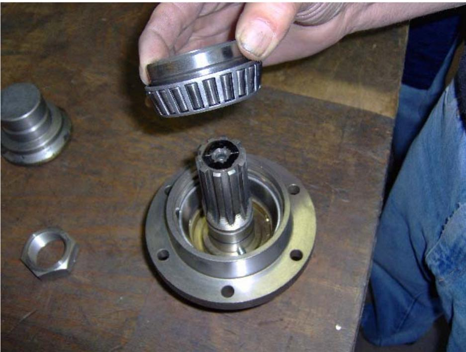
Put on the previously assembled shaft internally to the bearing housing.
