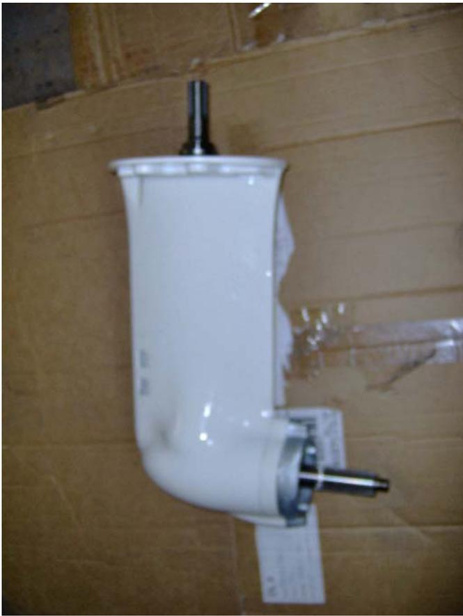
Manually check the shaft spin and the play between the tapered pairs. There should be no crawling during the spinning
