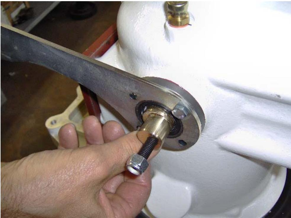
Put in the fixing screws (ref. n° 88) with thread locker, and tighten.
