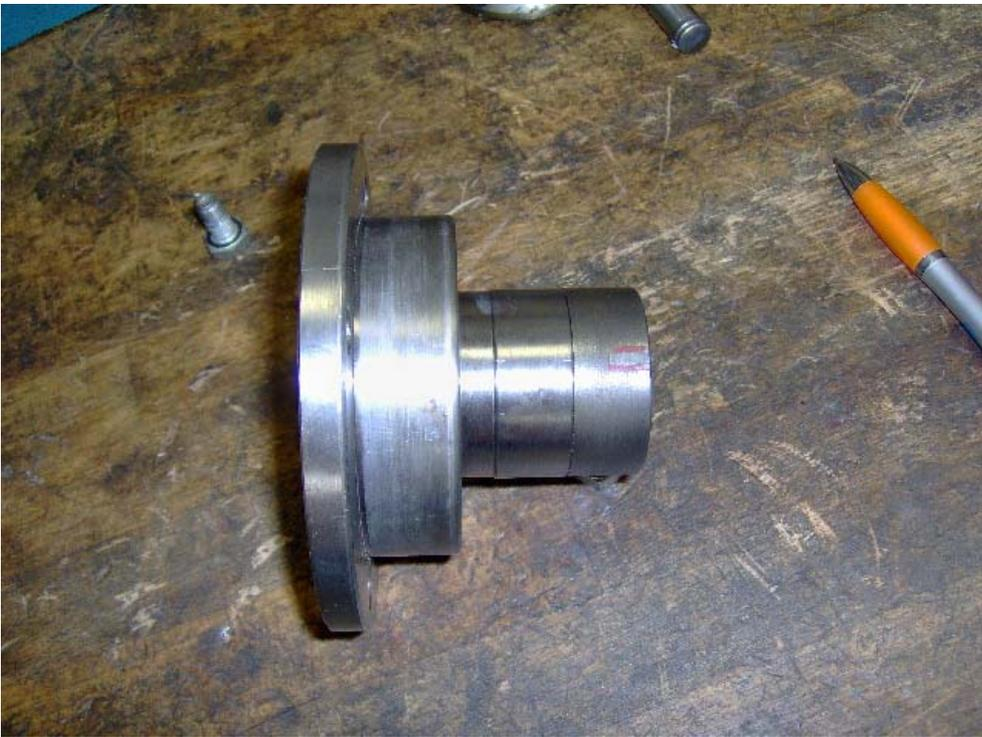
Insert and screw the centering tooling (tool SP60-08) as shown by scheme n° 3
