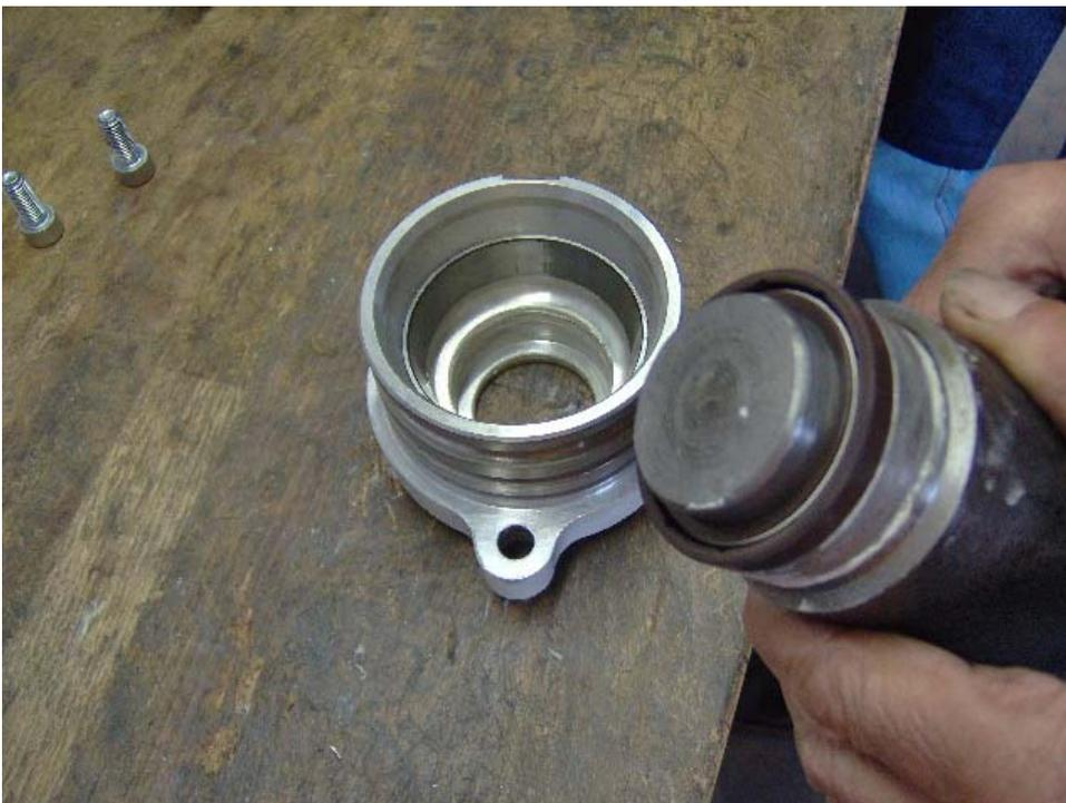
Put oil seals (ref. n° 79) in the support (ref. n° 78) as shown by the cross section drawing. Assemble the O-rings (rif. n° 80) and grease their surface to make their assembly easier.
