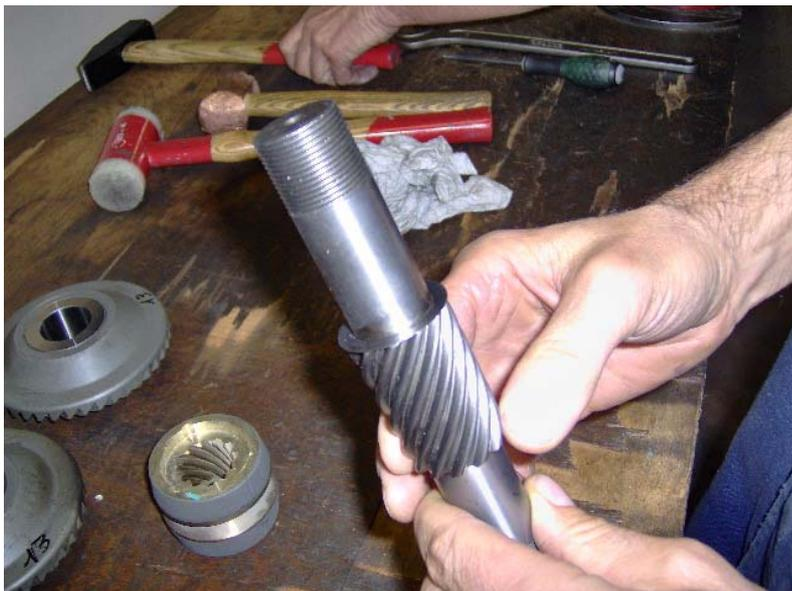
Put shim (ref. n°3) into the shaft (ref. n°1) until it hits the splined part of the shaft.
