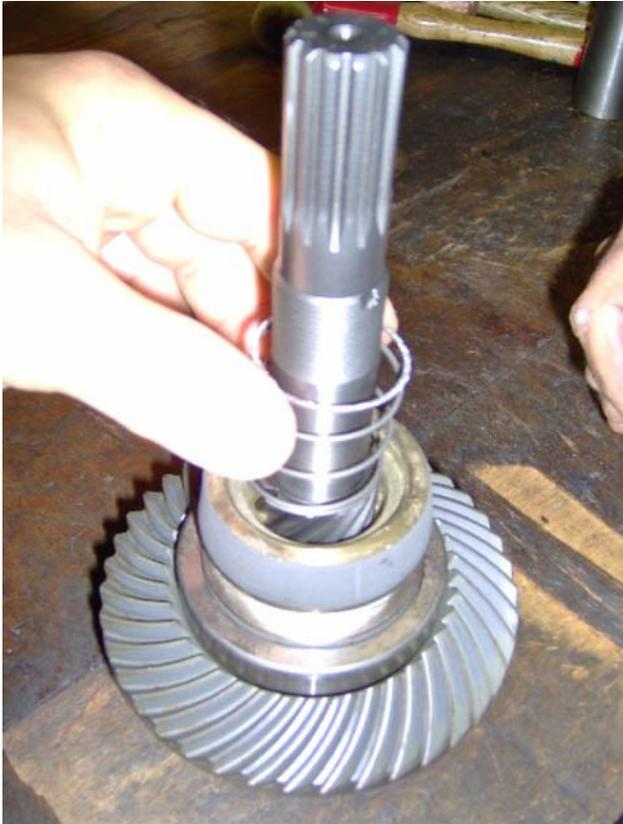
Put the clutch body (ref. n°2) into the shaft (ref. n°1), make sure it has enough play to the spline and it moves freely. Put on the opposition spring (ref. n° 12)
