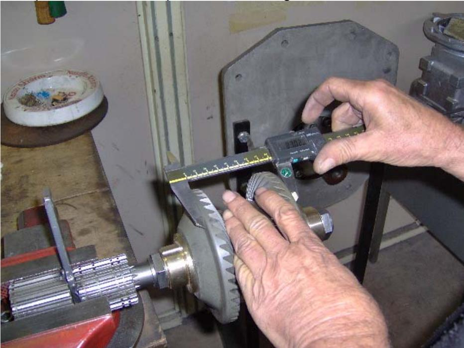
Measure the height of the clutch group, the value must be 83.02 mm.
