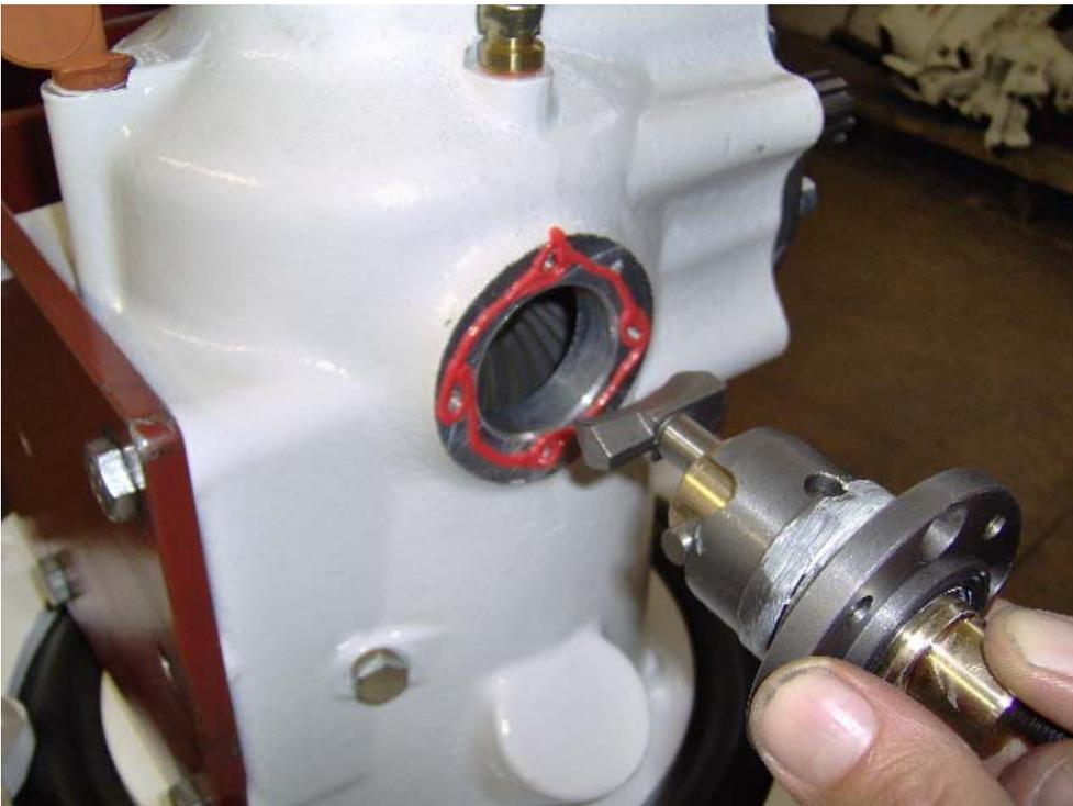
Apply layer of sealant paste as shown by the picture, insert the drive group previously assembled
