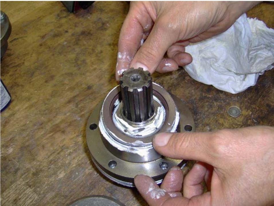
Put the oil seal (ref. n° 25) in its position, adding grease in its location to make the assembly easier.
