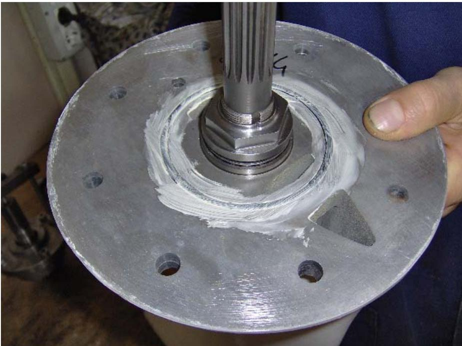
Put the o-ring ( rif. n° 65) in its location, apply grease to make the assembly easier
