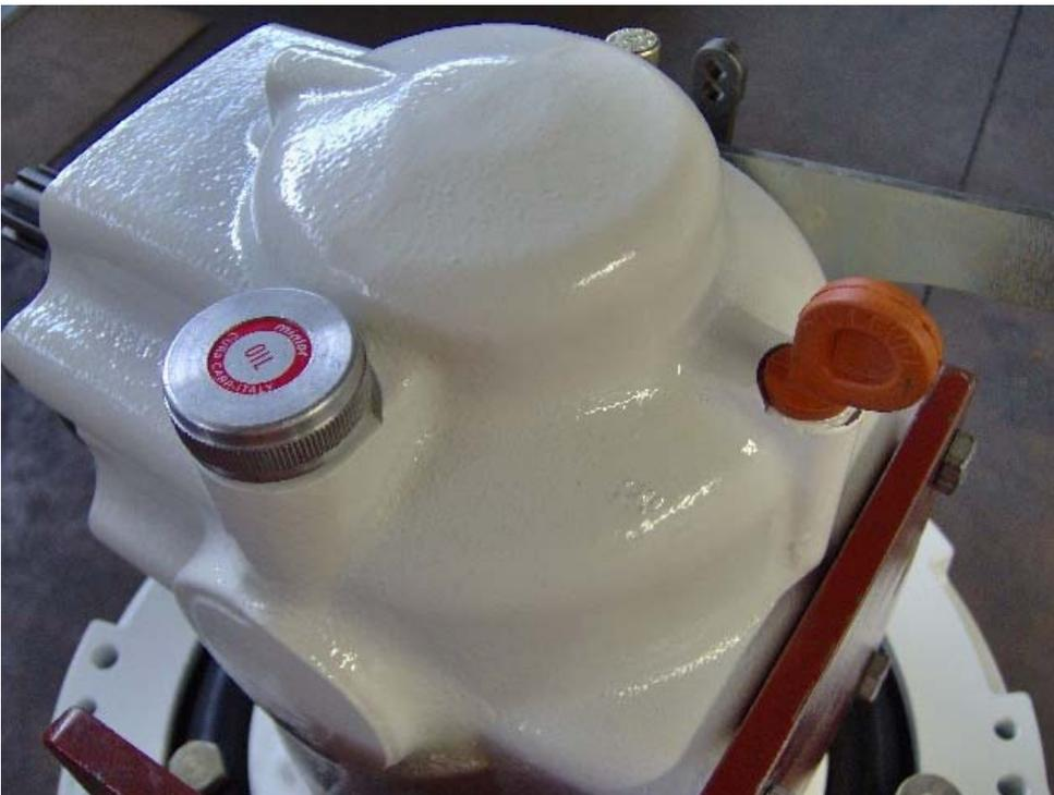
Finish the upper part of the gearbox, applying the oil dipstick and the oil filling plug. Apply and tighten the lock plug on the membrane( rif. n° 44)
