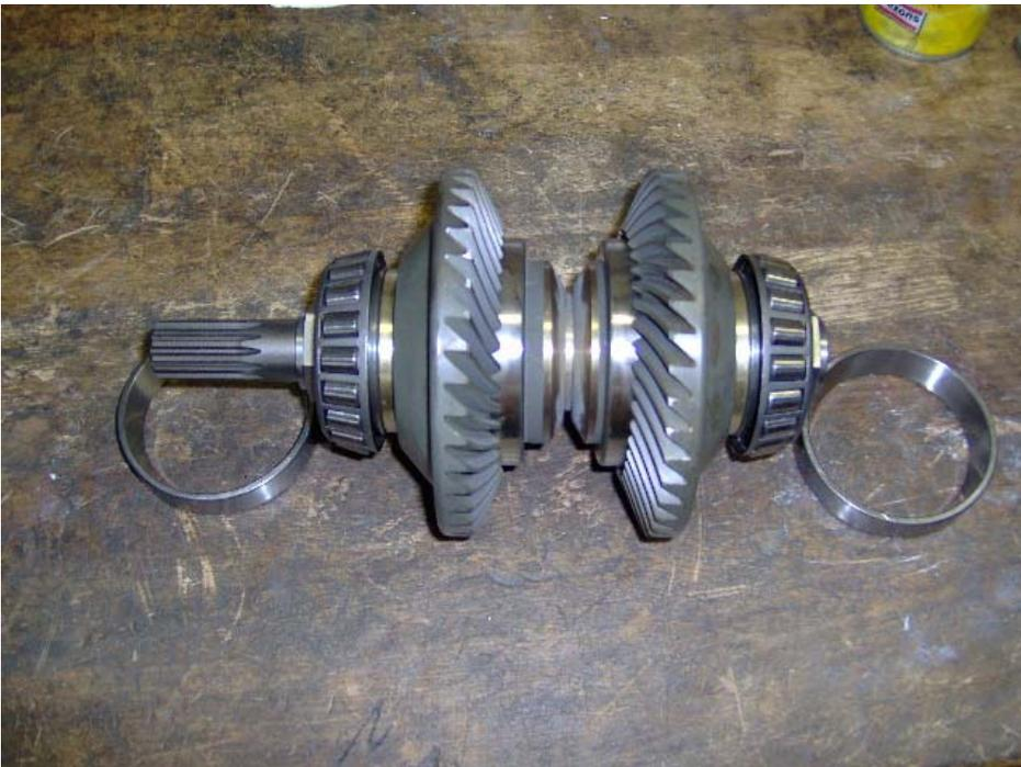
Position the preassembled clutch group with the thrust blocks of the respective bearings
