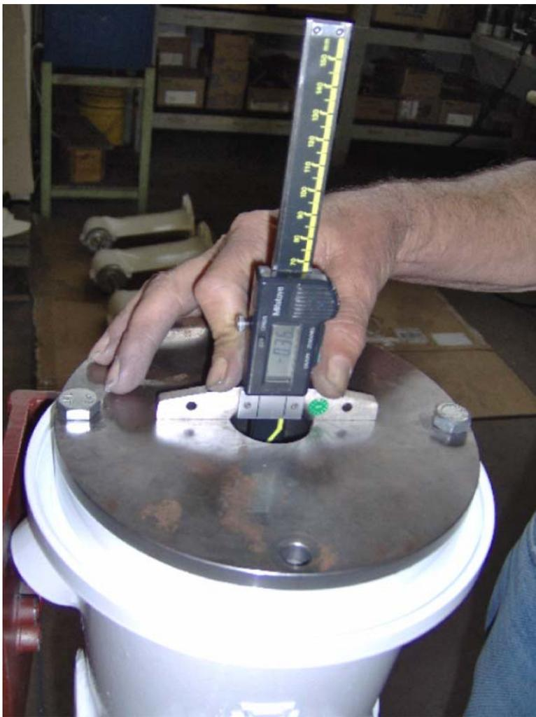
Verify the measurement on the top of the shaft with a depth gauge.
