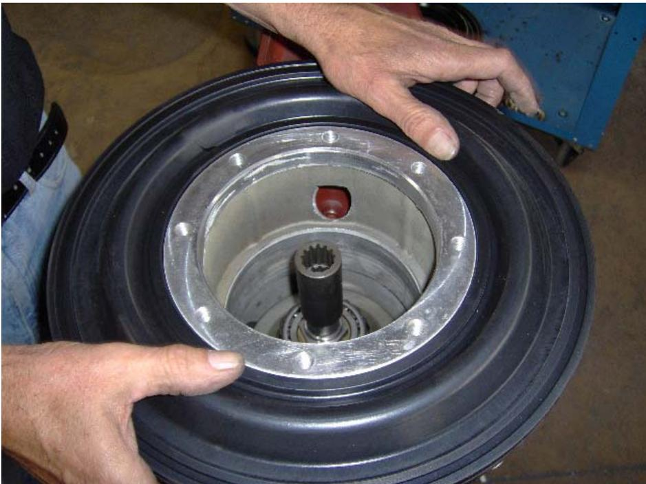
Insert the preassembled clutch group.
