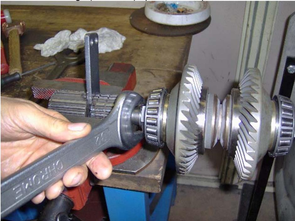
Screw the fixing nuts (ref. n°9), tighten and rivet the thread with a punch, in the position of the markings on the thread.
