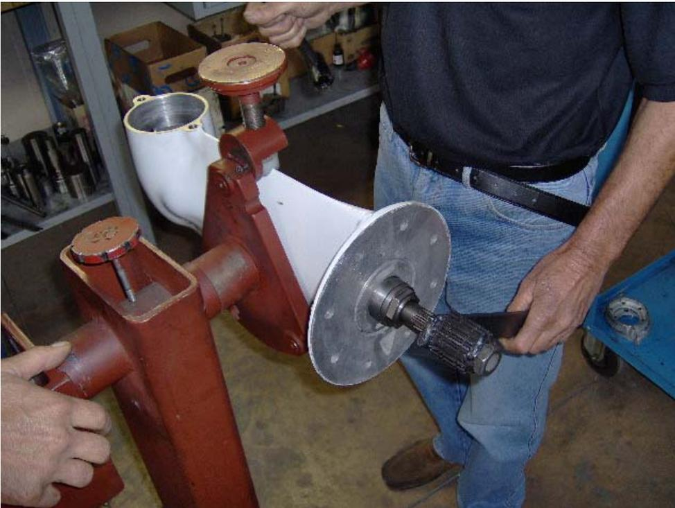
With the proper tool (tool SP60 -07), hold steady the shaft in order to prevent its spin, screw lock nut ( rif. n° 70) and ( rif. n° 61)
