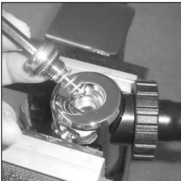
**Photo 1** HP Balance Plug Assembly removal
