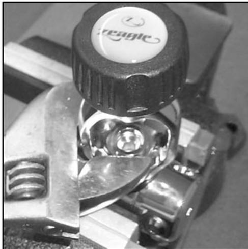
**Note:** If the regulator has a DIN wheel, use a 1/4" Allen wrench to remove the DIN bolt (21), and DIN wheel (24). The Flathead-VI also has a spacing washer (45) behind the DIN wheel.
