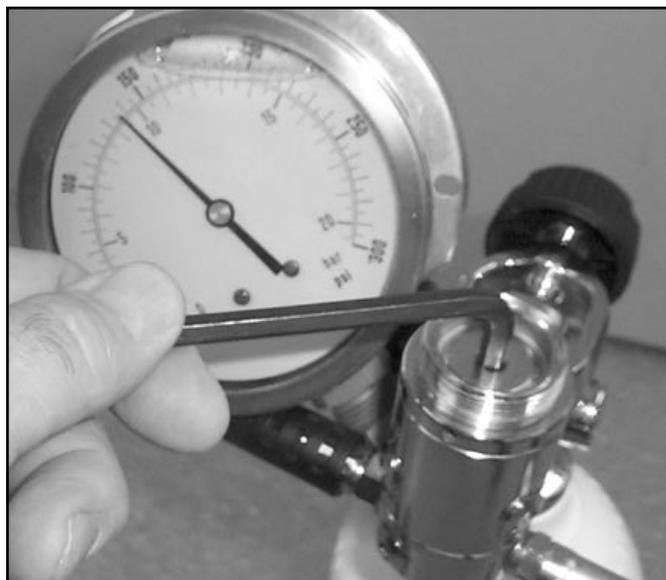
4.5.7 After reaching the proper pressure setting, push the purge cover on the second stage again several times and watch how the intermediate pressure reading responds. When the purge cover on the second stage is depressed, the intermediate pressure reading will drop. When the purge cover is released the pressure should return immediately to the proper lock-up pressure and stay there.
