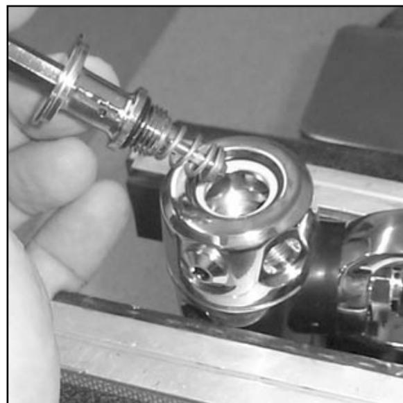
**Photo 2** Turret Bolt Assembly removal
