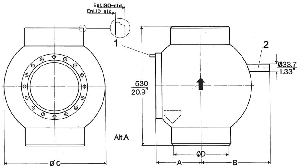
Pipe diameter ØD according to Inner Diameter (ID) metric standard or ISO standard. See section 8.3 for detailed measures.
