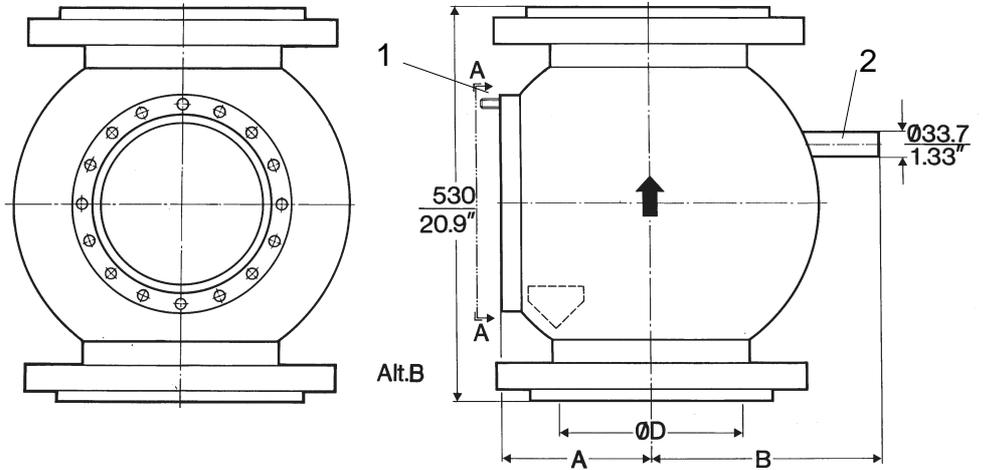
**Fig 21 Measuring vessel flanged on two sides for consistency transmitter and sampling valve type HDS.**
