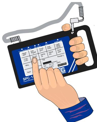
When the terminal is not in the wall terminal holder, place it on your left forearm (for right-handed users) and hold it securely using the hole in the handle. This is the best and safest way of using it, you can work properly without damaging the terminal.
