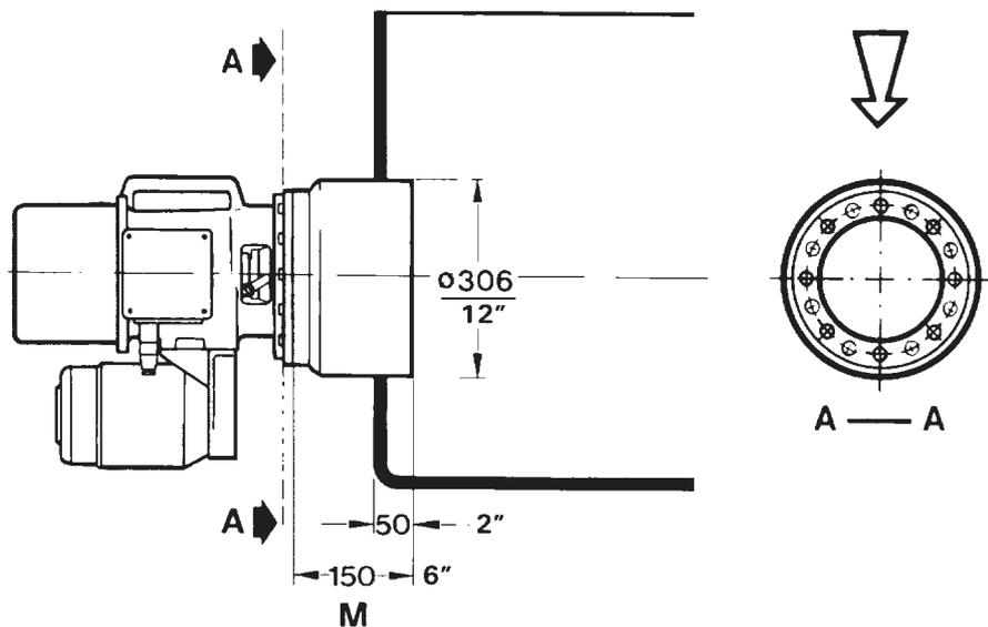
Fig 29 Example of level box for MEK-2340 — shaft length 700 mm / 27.5 in
