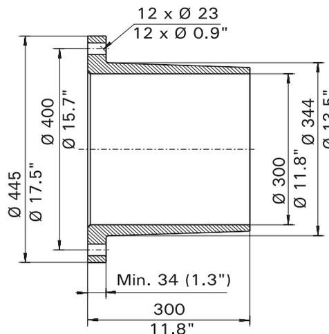
**Fig 27 Installation of Consistency Transmitter in FRP piping  $\geq 300$  mm (12 in) — low pressure**
