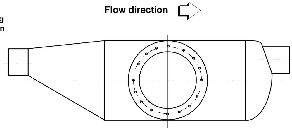
**Fig 12 Measuring vessel with stud for sampling valve — available to order**
