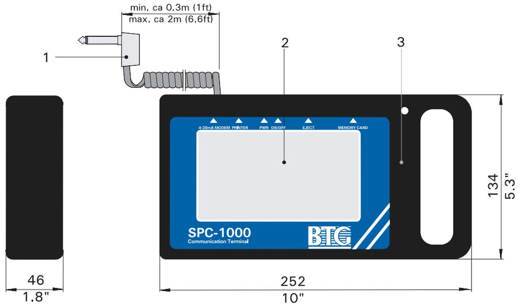
**Fig 4 Adapter for terminal connection (included with SPC-1000 delivery)**
