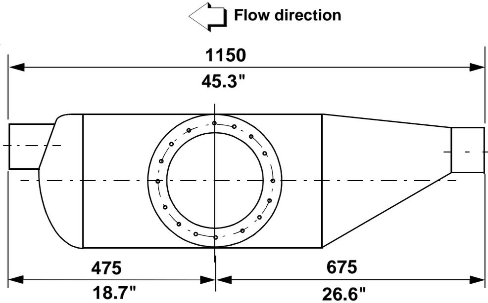
**Fig 11** Measuring vessel with weld-ends for low pressures and horizontal mounting — right-hand design (on request)
