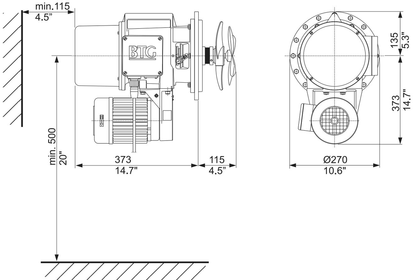
The transmitter, including sensor and propeller, is approximately 490 mm (19.5 in) long. In addition to the installed length of the transmitter, which will be 375 mm (15 in), you will need a minimum of an additional 115 mm (4.5 in) for extracting the transmitter from the pulp line. Leave sufficient room around the transmitter to perform this task.
