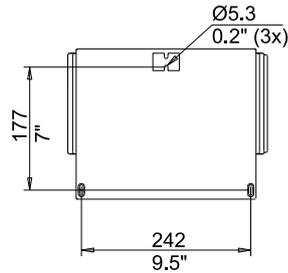
BTG recommends that a roof or overhang is mounted above the junction box to protect it against spray and pulp. If the junction box is located outdoors, a roof should be mounted that protects from direct sunlight which can cause excessive operating temperatures. If possible, the SPC-1000 should also be protected when placed in it's holder.
