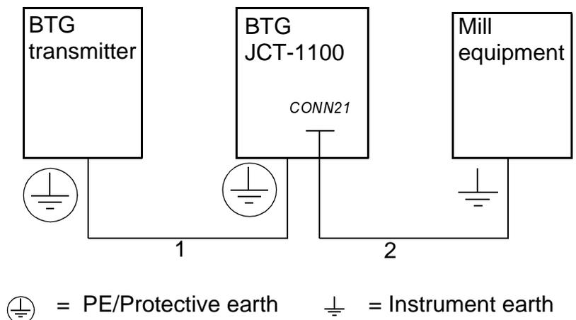
It is important to tighten the cable connector firmly to the transmitter – use a tool! If not tightened firmly, the shield will not be properly grounded.
