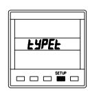
Press **SETUP** key to display the current mode.
