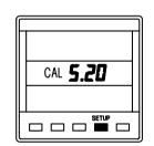
Press **SETUP** key three times to display **CAL**.
