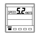
Press **SPEED** key to display current boat speed.
