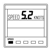
Press **SPEED** key to display the current boat speed.
