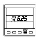
Press **SETUP** key four times to display **LOG CAL**
