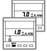
Press DEPTH key to display the anchor alarm.
