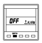
Press **DEPTH** key to display anchor alarm.
