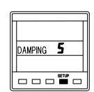
Press **SETUP** key once to display the damping value.
