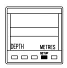
Press **SETUP** key twice. The depth display will go blank.
