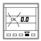
Press **SETUP** key to display current datum value. The display will flash.
