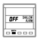
Press **DEPTH** key to display the shallow alarm.
