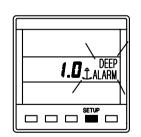
Press **SETUP** key 3 times to display the deep value.
