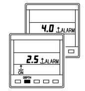
Press **DEPTH** key to display **ANCHOR ALARM**
