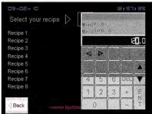
A soft keypad as shown in the screen on the right will appear. Here you can enter the desired recipe number within the range indicated on the top left of the soft keypad.
