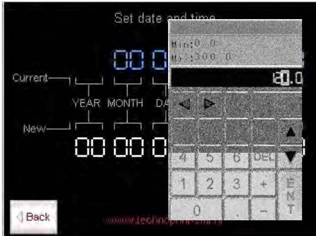
With the soft keypad appearing in the screen any number between 1 and 99 can be entered. Note that any number exceeding the maximum allowed value for the specific field entered will not be stored.
