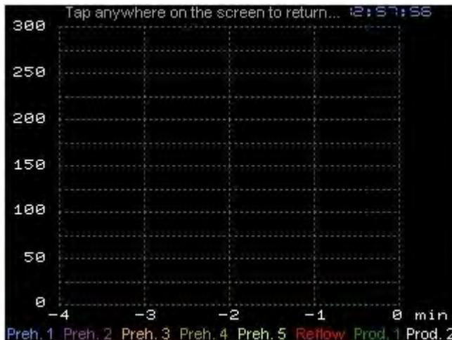
A screen like this will appear with graphs steadily changing for each temperature zone. When a thermocouple is connected a dotted line will appear indicating the probe's temperature.
