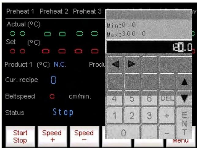
Setting the conveyor speed can be done as follows: Tap within the square with the conveyor speed setting. A soft keypad as shown on the left will appear on the screen. Entering a value for the conveyor speed is done in the same way as entering a value for the temperature. Settings entered both ways will always be saved after powering down the machine.
