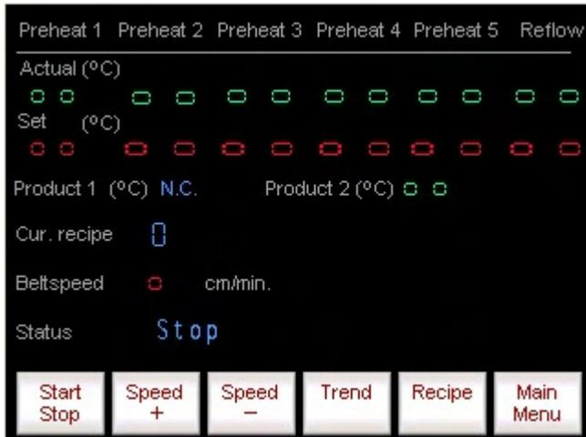
The profiling menu can be used to store, print or view important data registered by the thermo coupler(s).
