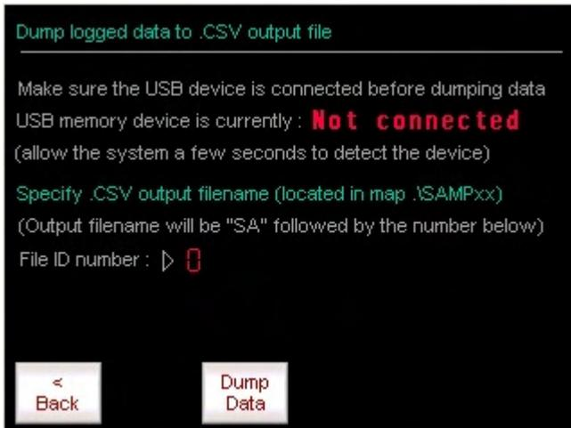
The next screen will indicate if USB storage is connected or not. Before data is dumped, a number can be assigned to the file by tapping on the “0” behind the file ID number.
