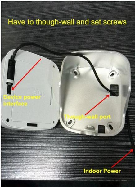
2) Second method power wire though bottom hole of holder for base, it's no need though-wall in this way, ref pic as following:
