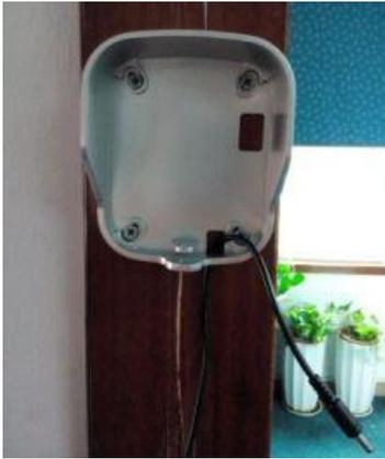
5.. Put doorbell unit on the holder of base, it's done after install disassembly-proof screw.
