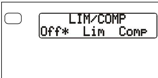
A **compressor** reduces, by a preset ratio, the level of any incoming signal which exceeds its preset level. For example, if your compressor is set for 10 dB and has a compression ratio of 2 to 1, any signal that comes in over 10 dB would be reduced by a factor of 2. For every 2 dB of input signal over 10 dB, the output level would only be increased by 1 dB. This is very useful when sending vocals, because they tend to have varying levels.
