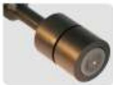
Please note that the black rubber seal is mounted on the sensor head and greased, than turn the cover on the sensor housing till it sturdily am stuck. Now the sensor is waterproof and can be installed in the probe holder.
