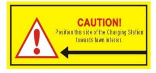
The charging station fence must face towards the interior section of the lawn when installed. Failure to do so may result in damage to property or persons.
