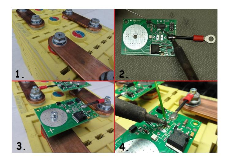
**WARNING:** be aware that your battery-pack contains a large amount of energy, which can be potentially lethal. Use isolated spanners, to prevent any short circuits. High inrush currents, causing arc-ing (sparks) and ultra-high electro magnetic levels, can easily damage electronic circuits.
