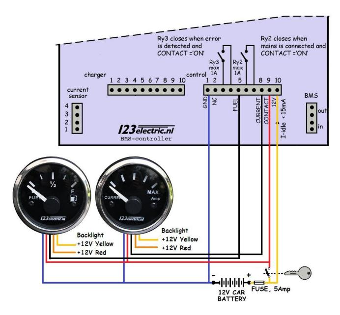
In the above schematic the 123Electirc current en fuel gauges are drawn. Might you want to use your existing fuel gauges for instance, you are free to do so. The BMS controller mimics a variable resistor between 0 and 240 Ohms and therefore practically any fuel gauge can be used. With the help of "analog gauge calibration" in the 123Electirc software you should be able to linearize the reading of your gauge.
